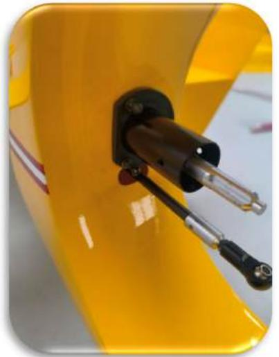
Then install the ball link onto the servo lever, and secure the fenestron tail frame on the tail boom, with the center screw and both tube clamps.
