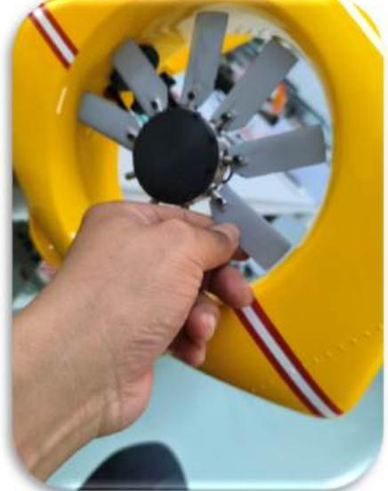
Then, adjust the fenestron (make sure the mechanic in the front can also move) so that it runs centered inside the duct as shown.
