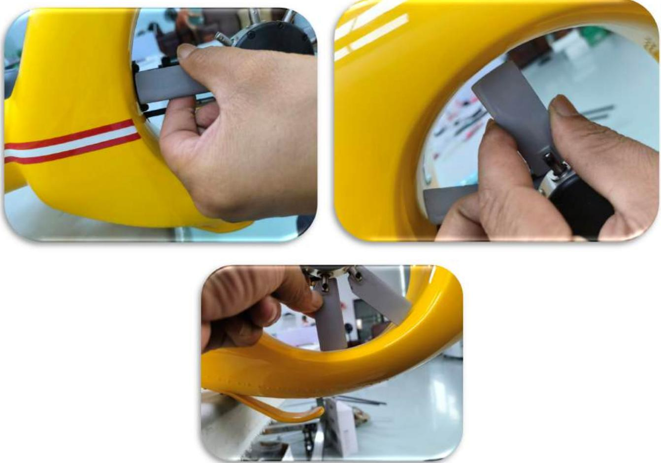
Once the fenestron is properly adjusted, start by tightening the three screws on the holding plate, and then proceed to tighten the clamp screws inside the fuselage through the access holes, as shown. Finally mount and tighten the tail boom to the front fuselage.
