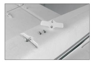
Insert the landing gear into its location, then lock it with the locker and screws to loosening.
