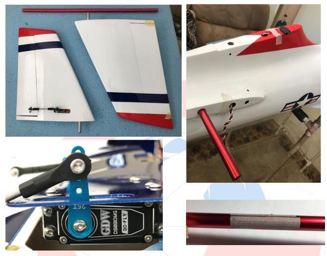
[] Disconnect the servo linkages from the horns on the elevators.
