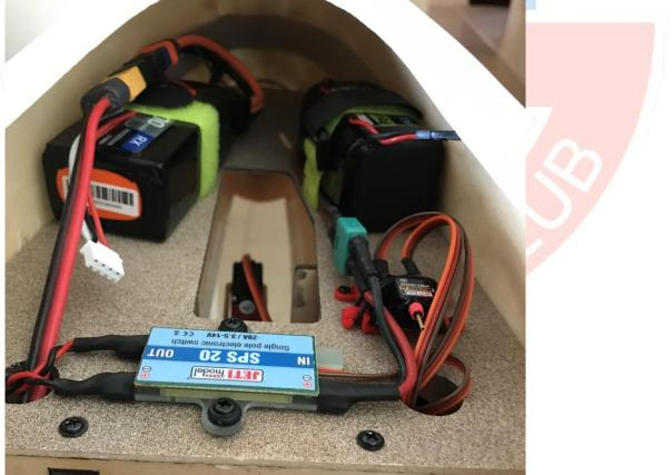
Once satisfied with your arrangement, install your systems. The forward board with batteries can go in last. All of the cables are long enough to be routed and plugged in with the main board out of the fuselage.
