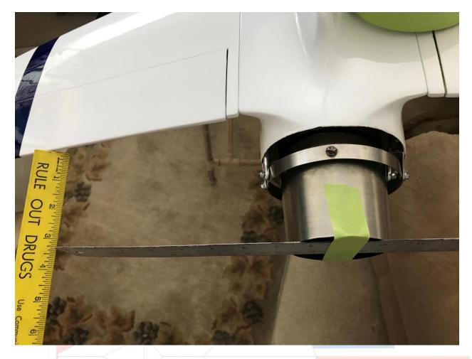
[] The linkage on yaw push rod may not be very tight inside the pushrod and the pushrod could easily rotate. This will prevent any trim changes or control rod linkages from disconnecting in flight. You may have to use CA to keep it from rotating. Check the pitch TV pushrod for the same condition.
