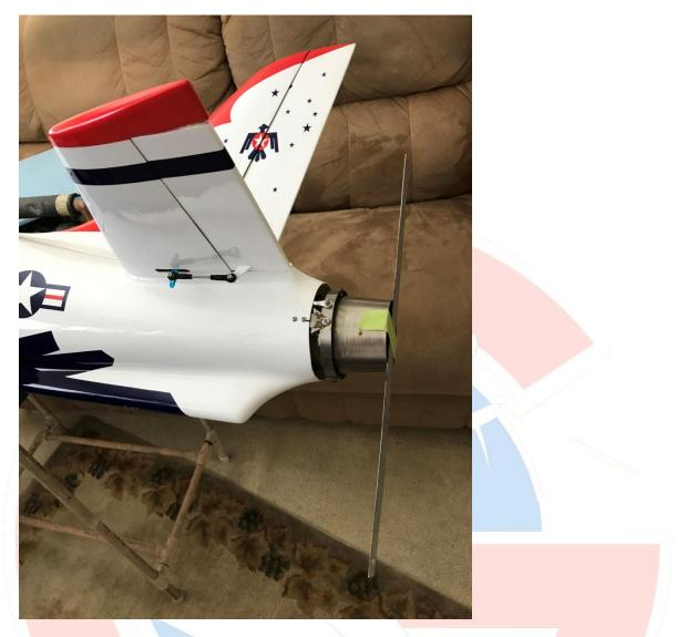
You may find some rubbing of the pitch pushrod in the back of the fuselage. We are flying as is and have not incounterred any issues
