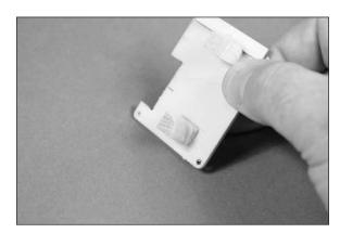
OO 15. Apply thin CA to the top of each servo mounting block. The wood fibers will soak in the CA, which will help prevent the blocks from splitting when they are drilled for the servo mounting screws.
