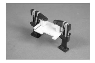
OO 13. Position the servo between the servo mounting blocks. Use a pencil to mark the block against the servo lead so it can be trimmed to provide clearance for the servo lead.
