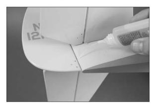
15. Gently pull on the fin and rudder to check that the hinges are glued securely. If you find any loose hinges, apply thin CA to the hinge to secure its location.
