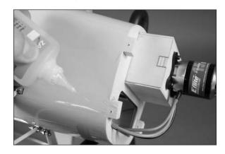
13. Use four 2mm x 8mm sheet metal screws to secure the cowling to the fuselage. Tighten the screws using a #1 Phillips screwdriver.
