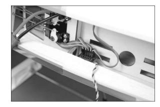
5. Use scissors to cut a small piece of hook and loop tape sized to fit the remote receiver. Use the hook and loop tape to mount the remote receiver forward and inside the fuselage as indicated. Note the direction of the antenna for the remote receiver.
