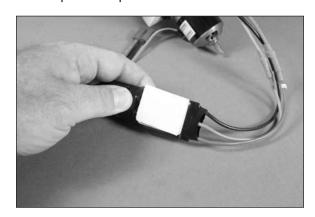
O 6. Insert the speed control into the opening in the front of the fuselage. Use the hook and loop tape to secure the speed control inside the fuselage.
