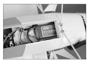
3. Replace the battery hatch on the fuselage.
