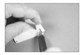
11. Use a sanding block or razor saw to remove the material necessary from the block to fit over the tab when the block is positioned on the cover for mounting the servo.
