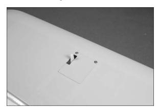
23. Insert the 4-inch (102mm) pushrod wire into the hole in the servo horn enlarged in Step 20. Use a nylon pushrod connector to secure the pushrod to the servo horn. You may need to use pliers to snap the connector over the wire.
