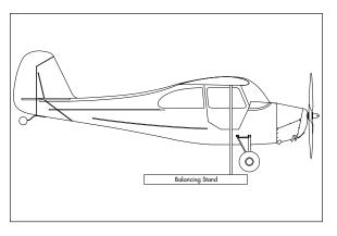
Adjust the motor battery as necessary so the model is level or slightly nose down. This is the correct balance point for your model. You should find the CG to be very close with the battery installed as shown in this manual. Mark the location of the battery on the battery tray using a felt-tipped pen so it can be returned to this position if it is removed from your model.
