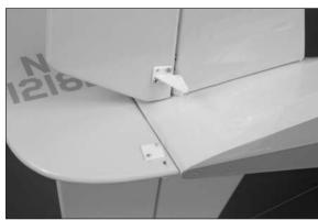
4. Slide the 19<sup>7</sup>/<sub>8</sub>-inch (505mm) rudder pushrod into the guide tube in the fuselage. You may need to assist it exiting the rear of the fuselage so it doesn't damage the covering at the exit.
