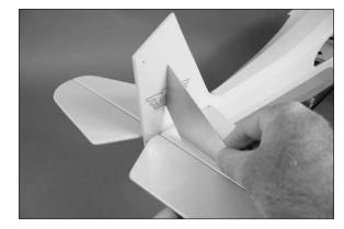
**Note**: Because the covering is flared near the base of the fin, you will need to use a square that is notched as shown in the photo, or measure the angle as close to the hinge line as possible to avoid the covering interfering with checking the alignment.
