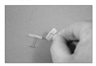
11. Place the hinges in the slots in the fin. The hinge that does not have a T-pin is located at the top of the fin as it will only slide in partially due to the hardwood block installed in the fin for the tail rigging.
