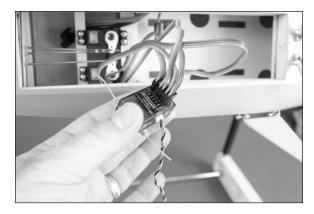
**Note**: Use a Y-harness for both aileron leads when using a non-computer radio without the capability of individual aileron channels. Plug the Y-harness into the aileron port of the radio.
