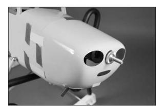
O 11. Use a pin vise and 1/16-inch (1.5mm) drill bit to drill the four holes for the cowl mounting screws. Use the card stock in locating these screws.
