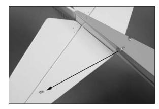
5. Tie the rigging line to the fitting on the fin. We recommend using tweezers or hemostats to hold onto the line while tying the knot. Once tied, place a drop of thin CA on the knot to keep it from coming loose.
