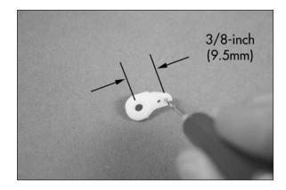
8. Use a #1 Phillips screwdriver to remove the stock servo horn from the servo. Install the servo horn prepared in Step 6 on the servo. Note the position of the servo horn for the rudder and elevator servos.
