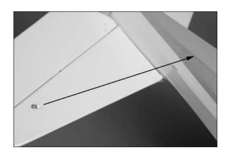
3. Attach a pair of rigging fittings to the rudder using a 2mm x 8mm machine screw and a 2mm nut. Make sure the small hole in the fitting faces in the direction of the fittings on the top of the stabilizer. Use a #1 Phillips screwdriver and 4mm nut driver to tighten the hardware. Do not fully tighten the nuts at this time.
