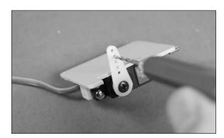
21. Tie the end of the string in the servo opening to the end of the servo extension.
