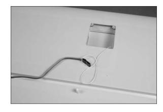
21. Use the string to pull the servo lead and extension through the wing and out at the wing root as shown.
