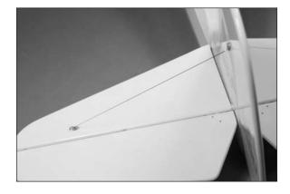
8. Tie the rigging on the bottom from the stabilizer to the fuselage. Again, use hemostats or tweezers when tying the knots, and apply a drop of thin CA on the knot to prevent it from coming loose. Fully tighten all of the nuts and screws on the rigging at this time using a #1 Phillips screwdriver and 4mm nut driver. Use thin CA on the outer side of each nut to hold them in place.
