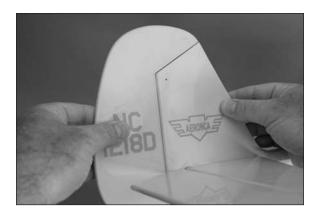
16. Flex the control surface through its range of motion a number of times to break in the hinges.
