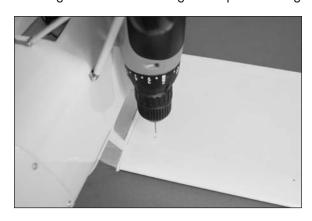
OO 5. Use a #1 Phillips screwdriver to install the 2.6mm x 10mm sheet metal screw that holds the tube in the wing panel. Use care not to strip the head of the screw during its installation as you are tapping the aluminum tube to fit the screw. Remove the tape from the tube on the other side.
