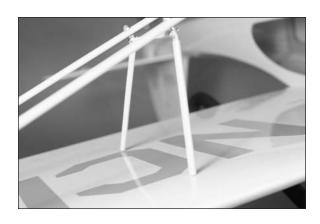
15. Repeat Steps 2 through 14 to install the remaining wing strut.
