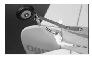
O 6. Repeat Steps 3 through 6 to prepare and install the remaining tail wheel spring.
