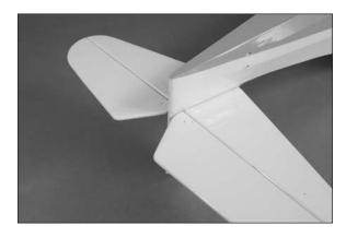
O 6. Use a straight edge to check that the hinge lines between the right and left stabilizer are aligned with each other. You won't be able to fit the straight edge right to the hinge line, but you can measure from the hinge line to the straight edge for alignment.
