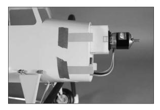
9. Slide the cowl in position on the front of the fuselage. Make sure the card stock is on the outside of the cowl.
