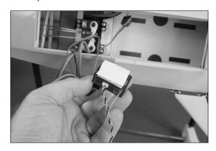
4. Use the hook and loop tape to secure the receiver in the fuselage. Make sure the antennas on the receiver, are straight. If they are not straight, it could reduce the range of the radio system. Carefully tuck the servo leads so they don't interfere with the operation of the rudder and elevator servos.
