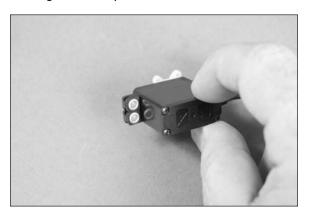
7. Locate the standard servo horn included with your servo. Use a pin vise and 5/64-inch (2mm) drill bit to enlarge the hole in the servo arm that is 3/8-inch (9.5mm) from the center of the horn. Use side cutters to remove any unused arm from the horn so they don't interfere with the operation of the servo.
