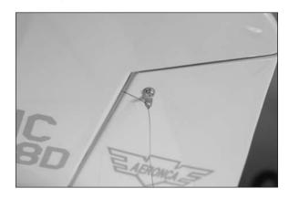
OO 6. Tie the rigging at the fitting on the top of the stabilizer. Use hemostats or tweezers to hold the line while tying the knot. Place a light amount of tension on the line. Make sure not to pull the stabilizer out of alignment with the fin, so use a square to verify the stabilizer and fin are still aligned. Once tied, place a drop of thin CA on the knot. Use scissors to trim the excess line as close to the fitting as possible.
