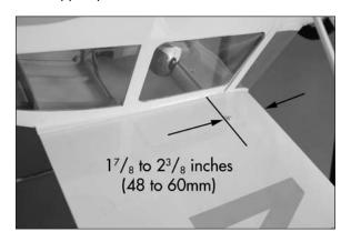
5. When balancing your model, support the plane upright at the marks made on the bottom of the wing with your fingers or a commercially available balancing stand. This is the correct balance point for your model. Make sure your model is assembled and ready for flight before balancing.
