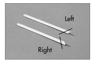
7. Insert the bend in the wing strut supports in the wing with the support facing the fuselage. Carefully lift the strut support into position so it is perpendicular to the wing. Note that the longer support is located near the trailing edge of the wing. Insert both the long and short supports at this time.
