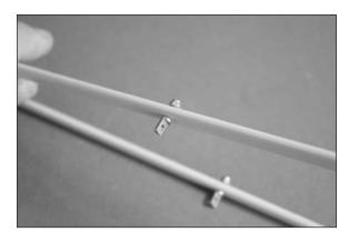
10. Locate the nylon strut fittings. Carefully bend the fitting slightly once along the embossed line. Repeated bending can damage the fitting and may cause it to fail in flight. Prepare two fittings at this time.
