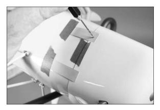
O 12. Remove the propeller adapter, cowling, card stock and tape from the fuselage. Apply 2–3 drops of thin CA in each of the holes drilled to harden the surrounding wood. This will help prevent the screws from vibrating loose in flight.
