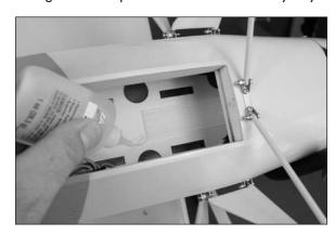
2. Apply the mating surface of the hook and loop tape to the battery. Install the battery into the compartment.
