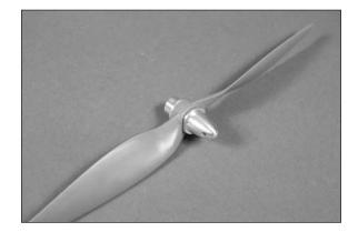
O 15. Slide the propeller assembly on the motor shaft. Use a 3/32-inch hex wrench to tighten the adapter nut, securing the propeller assembly to the motor shaft.
