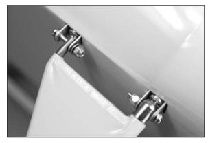
5. Secure the strut leg from the landing gear to the bottom landing gear mount using a 2mm x 12mm machine screw, two 2mm washers and a 2mm locknut. Use hemostats to hold the locknut while tightening the screw using a #1 Phillips screwdriver. Do not over-tighten the screw and cause binding of the landing gear.
