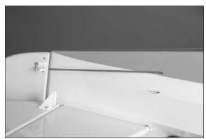
O 5. Slide a silicone clevis retainer over a nylon clevis. Thread the clevis 10-turns on the end of the rudder pushrod. Connect the clevis to the outer hole of the rudder control horn. The overall length of the pushrod must still be adjusted, so don't slide the retainer over the clevis at this time.
