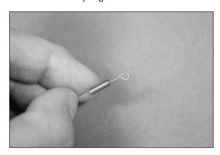
4. Make a second loop in the spring using pliers. The overall length of the spring will be 1-inch (25mm) as shown. Use side cutters to trim any excess wire.
