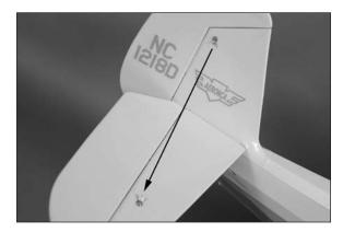
4. Install the last two fittings on the bottom of the fuselage using 2mm x 6mm sheet metal screws. Make sure the fittings are directed toward the fittings on the bottom of the stabilizer. Use a #1 Phillips screwdriver to tighten the screws. Do not fully tighten the screws fully at this time.
