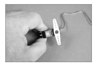
7. Position the servo on the cover, using the lines drawn in Step 5. Adjust the position of the servo so the servo horn is positioned center in the opening as shown.
