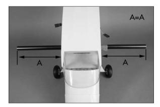
OO 2. Slide a wing panel on the wing tube on the side without the tape. Make sure to connect the extensions from the wing and fuselage.
