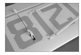
○○ 14. Insert a 2mm x 5mm machine screw in the support cross brace. The screw then goes through the support and threads in the fitting. Tighten the screw using a #1 Phillips screwdriver. Use two screws to secure the front and rear supports to the fittings.
