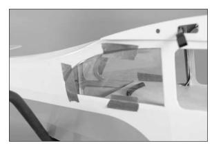
Repeat Step 1 to secure the side windows in the fuselage.
