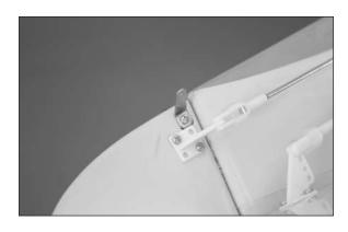
Attach the tail wheel assembly to the bottom of the fuselage using two 2mm x 8mm sheet metal screws and a #1 Phillips screwdriver.
