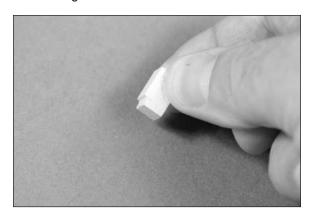
12. Use 6-minute epoxy to glue the servo blocks to the servo cover. Use clamps to hold the blocks in position until the glue fully cures.
