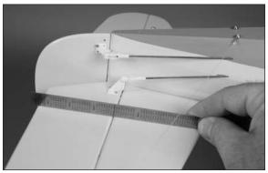
O 17. Adjust the position of the clevis on the rudder pushrod so the balance tab on the rudder is aligned with the fin when the clevis is connected to the control horn. Once adjusted, slide the silicone clevis retainer over the forks of the clevis to keep it from opening accidentally in flight.
