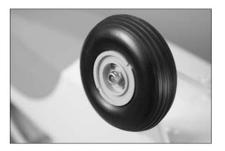
OO 9. Place the hub cap back in position to complete the wheel installation.
