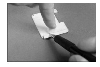
10. With the block positioned on the marks made for the servo, use a pencil to mark the block for the amount required to be removed so it can fit over the tab.
