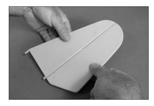
2. Flex the control surface through its range of motion a number of times to break in the hinges.
