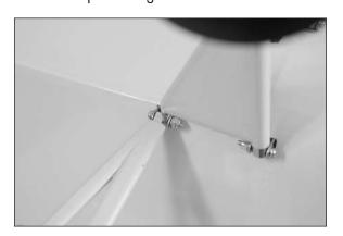
13. Position the nylon strut fittings and check that they fall naturally over the holes in the wing. If not, readjust the fittings so they do. Use two 2mm x 8mm sheet metal screws and a #1 Phillips screwdriver to secure the strut fittings to the wing.
