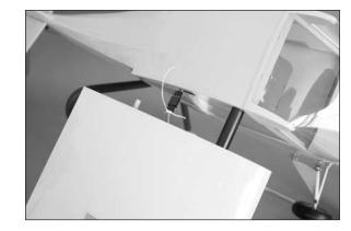
OO 3. Slide the wing tightly against the fuselage. Check to make sure the wing tube has not slid out of position. If so, reposition the wing tube so the tape is against the fuselage.
