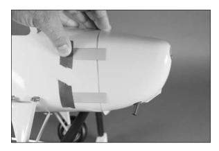
O 10. Slide the propeller adapter in position on the motor shaft. Slide the cowl rearward so the propeller adapter can rotate without rubbing on the cowl. Align the cowl so the propeller adapter is centered in the opening. Use low-tack tape to hold the cowl on the fuselage.
