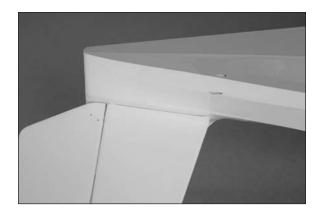
5. Repeat Steps 3 and 4 to position the remaining stabilizer. The dowels from the right and left stabilizer will fit against each other in the stabilizer tubes in the fuselage.
