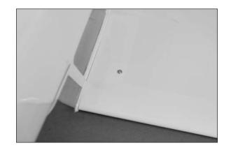
O 6. Locate the long wing strut supports. Note that there is a right and left support, which are differentiated by the angled cut near the L-bend in the wire. Make sure to install these in the correct wing panel. Note that left and right are viewed as if sitting in the pilot seat.
