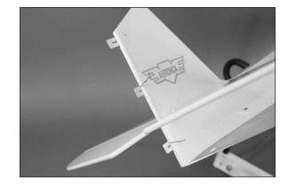
12. Position the rudder on the fuselage and fin. Remove the T-pins from the hinges. There should be no gap between the rudder and fin along the hinge line.
