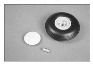
OO 8. There is a brass spacer located inside the wheel. Make sure this spacer is installed in the wheel before placing the wheel on the axle or it will not roll correctly. Slide the wheel on the axle. Use a 4mm locknut and 7mm nut driver to tighten the nut. Do not over-tighten the nut so the wheel can roll freely.
