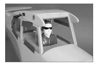
6. Test fit the front windscreen into position. Once fit, apply canopy glue around the perimeter of the windscreen where it contacts the fuselage. Use lowtack tape to hold the windscreen in position until the glue fully cures.
