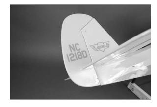
13. Check the gap between the rudder balance tab and top of the fin. There should be just enough clearance to allow the rudder to move without binding on the fin.
