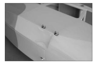
3. Attach the bottom landing gear mount to the bottom of the fuselage using two 2.6mm x 10mm sheet metal screws. Use a #1 Phillips screwdriver to tighten the screws.
