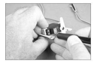
17. Use a pin vise and 1/16-inch (1.5mm) drill bit to drill the holes in the servo mounting blocks for the servo mounting screws.
