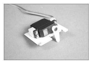
20. Use a pin vise and 5/64-inch (2mm) drill bit to enlarge the hole on the servo horn that is 11/16-inch (17.5mm) from the center of the servo horn.
