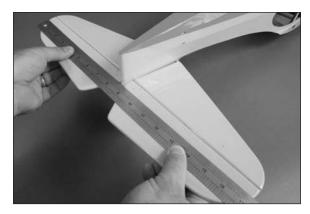
7. Use a straight edge to check that the stabilizers are parallel with each other as well. Although this can be corrected slightly when installing the tail bracing, it is best to try and set this alignment as close as possible at this time.
