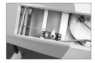
15. Repeat Steps 4 through 14 to install the 19-inch (482mm) elevator pushrod.
