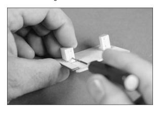
18. Apply 2–3 drops of thin CA in each hole to harden the surrounding wood. This will help keep the screws from vibrating loose.
