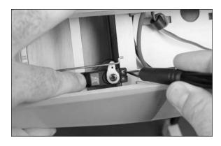
11. Remove the servo from the servo tray. Use a pin vise and 1/16-inch (1.5mm) drill bit to drill the four holes for the servo mounting screws.
