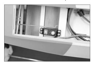
14. Disconnect the clevis at the rudder control horn. Insert the bend in the rudder pushrod in the hole enlarged in Step 6 for the servo horn. With the rudder servo centered, attach the servo horn on the servo so it is perpendicular to the servo centerline. Install the screw securing the horn to the servo using a #1 Phillips screwdriver.
