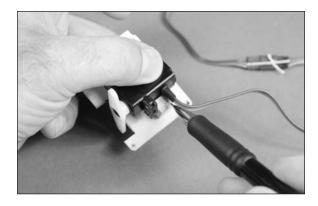
14. Use a razor saw and sanding block to trim the servo mounting block to allow clearance for the servo lead.
