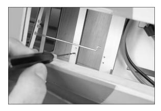
12. Apply 2-3 drop of thin CA in each of the holes to harden the surrounding wood. This will help in preventing the screws from vibrating loose.
