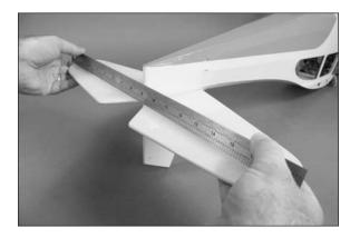
8. The final alignment check is to make sure the stabilizers are perpendicular to the fin. Use a square to check this on both the right and left stabilizer halves.
