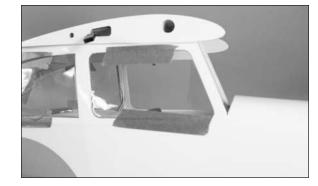
O 3. (Optional) If you are installing the optional pilot, use medium CA to assemble the pilot.
