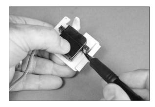
9. Position the block on the cover near the rear of the cover. It will be necessary to notch the block to fit over the tab that secures the rear of the cover. Position the block against the tab and use a pencil to draw a line on the block to determine how much to remove.
