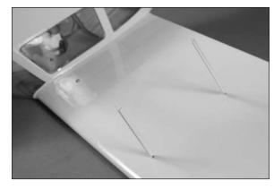
30 8. Locate the wing struts. The wider strut will face to the front of the airframe, while the narrow strut will face the rear of the airframe.
