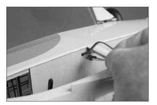
O 2. Use hemostats to retrieve the leads for the aileron servos and bring them up along side the rudder servo. Plug the 12-inch (305mm) extension into the aileron channel, the 9-inch (228mm) extension into the flap channel, and rudder, elevator and speed control into the correct ports of the receiver.
