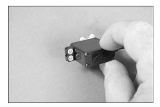
2. Connect a 6-inch (152mm) servo extension to the servo lead. Use scissors to cut a 3-inch (76mm) piece of string. Use the string to secure the extension to the servo.
