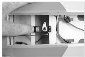
OO 10. Slide the rudder servo into position. The rudder pushrod will align with the hole in the servo horn enlarged in Step 6. Use a pencil to mark the location for the servo mounting screws on the servo tray.
