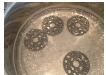
motor mount anealing in boiled water
