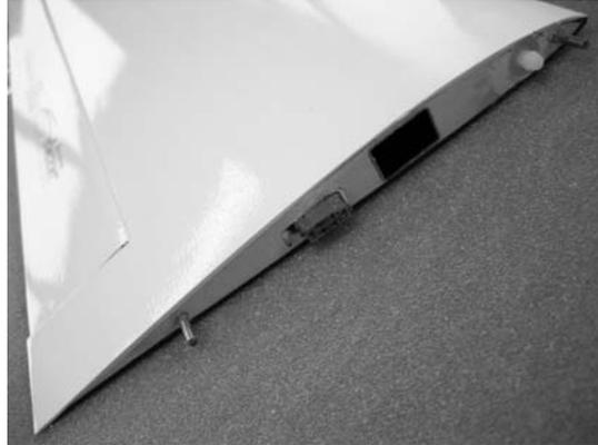
The four incidence pegs must now be glued in the wing root ribs so that the wings have a fixed location relative to the fuselage, and cannot swivel on the wing joiner.
