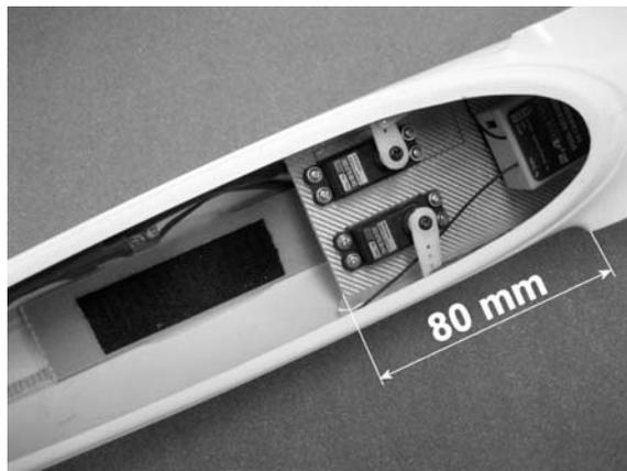
The flight battery can be fixed to the battery plate using Velcro (hook-and-loop) tape. Once you have established the correct Centre of Gravity, mark the battery's position using a pencil.
