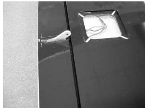
While the glue is curing you can use the time to cut down the servo output levers to the shape shown in the photo. Drill out the outermost hole in the output arm to 1.6 mm  $\varnothing$  to suit the threaded steel pushrod.
