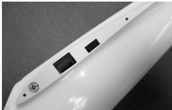
Drill 3 mm Ø holes in the wing root ribs for the incidence pegs, drilling to a depth of 50 mm. To check the fit, plug the two wing panels into the fuselage using the rectangular CFRP joiner and the incidence pegs. Take care not to push the steel dowels right into the wings.
