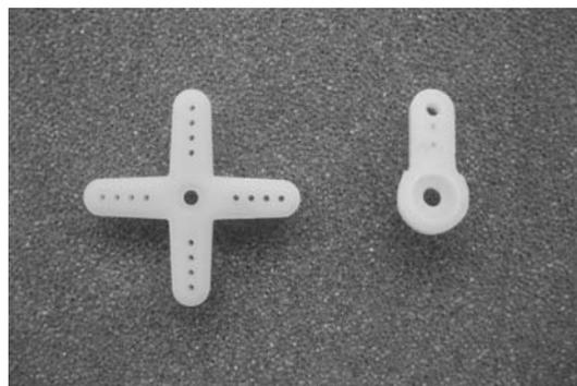
Centre the servos, then push the prepared output arms onto the servo output shafts and fit the retaining screws.
