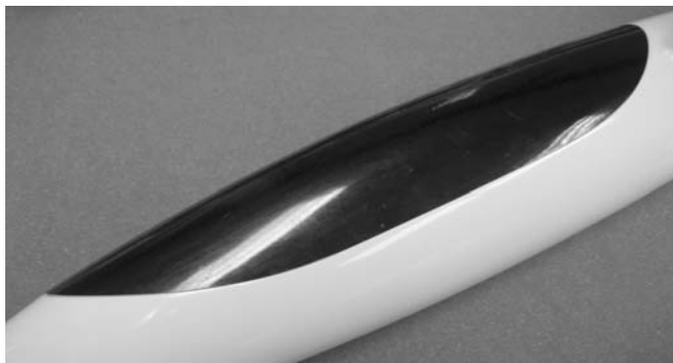
Before the RC plate is glued in the fuselage, the special peel ply on the inside of the fuselage sides must be removed as shown in the picture.
