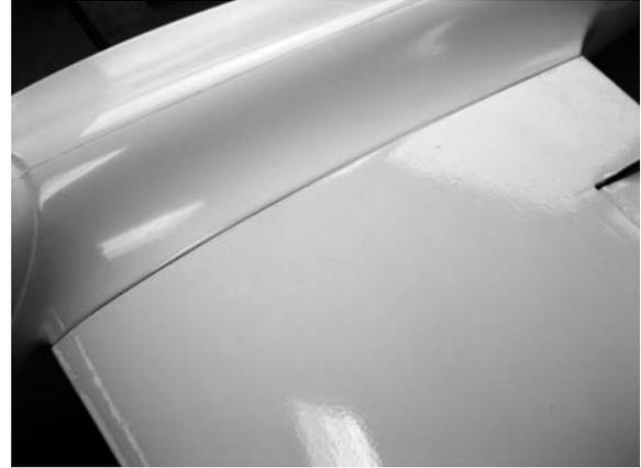
While the wings are plugged into the fuselage, please check that the tailplane lines up correctly with the wings. You will find a small compression strut in the wooden parts bag. Install this component between the wings close to the trailing edge, and adjust its position to correct any minor production tolerances in the wing sweep angle. It is important to epoxy the compression strut in place at this stage.
