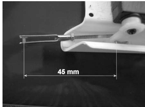
It is essential to apply a drop of UHU schraubensicher (thread-lock fluid) between the clevis and the locknut to prevent the clevis working loose.
