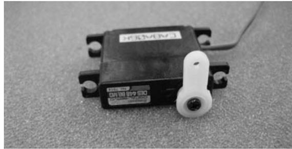
The next step is to glue the servos to the servo well covers, but first you will need to solder the servo leads to the extension leads (already present in the wings), and remove the servo mounting lugs. Solder the joints carefully, ensuring that you maintain correct polarity, i.e. connect like colours of wire together. Insulate each soldered joint with a separate heat-shrink sleeve, which must be fitted onto the wire before the joint is soldered.
