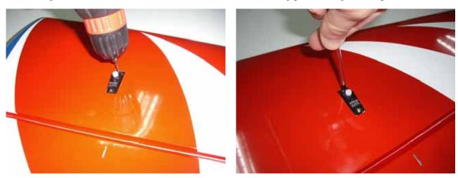
$\Box\Box$  step 4 Glue the fibreglass horn with medium CA into the aileron.
