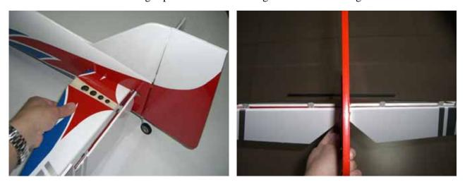
$\square$  step 4 Locate the elevator hinges into the stabiliser. Glue carefully the hinges in the stabiliser with some drops of thin CA.
