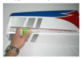
□□ **step 3** Locate the aileron and carefully glue, with some drops of thin CA, the hinges into the wing panel.
