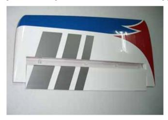
$\Box\Box$  step 2 Carefully glue, with some drops of thin CA, each of the four hinges in the aileron.
