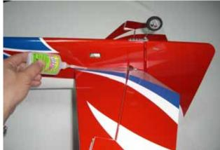
Section 5 – elevator servo & control horn installation
