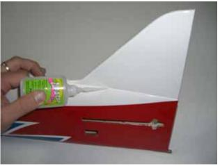
$\Box$  step 6 Insert the three hinges in their appropriate slots of the rudder, and glue them with some drops of thin CA.
