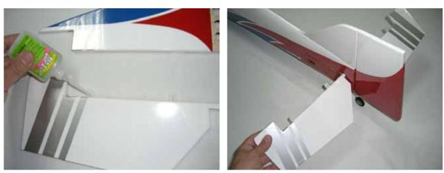
$\Box$  step 3 Insert the stabiliser into fuselage space and check the alignment with the wing carbon tube.
