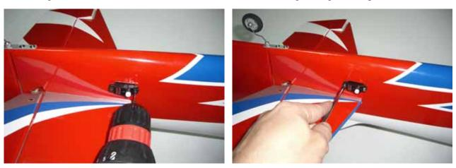
$\Box$  step 4 Glue the fibreglass horn with medium CA into the elevator. Than install the hardware and make the final adjustment as per picture.
