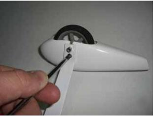
$\square\square$  step 3 Locate the landing gear on the fuselage and fix it with the 3 screws included in the hardware pack.
