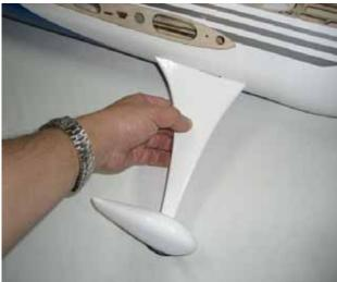
$\Box\Box$  step 5 Glue carefully the landing gear fillet with some drops of medium CA, as per picture.
