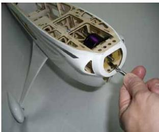
$\square$  step 2 Locate and fix the ESC and his switch as per picture.
