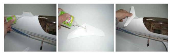
$\square$  step 3 Install on both wing panels the small deflectors, gluing the parts carefully with some drops of thin CA, as per pictures.
