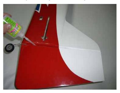
$\square$  step 8 Work the rudder right and left some times to work the hinges and check for proper movement.
