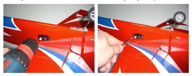
$\square$  step 4 Glue the fibreglass horn with medium CA into the elevator. Than install the hardware and make the final adjustment as per picture.
