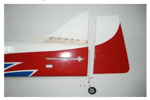
$\Box$  step 3 With the hobby knife cut a groove of 15mm length into the rudder. Drill in the rudder, 15mm from the bottom, the location for the tail wheel using a 2mm drill bit.
