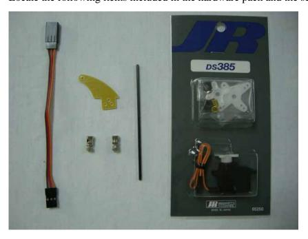
$\square\square$  step 2 Install the servo hardware (gommets and eyelets) and put the servo into the wing panel, as per pictures.
