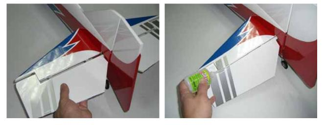
$\Box$  step 5 Once satisfied with the alignment, glue carefully with thin CA the stabilizer at the fuselage.
