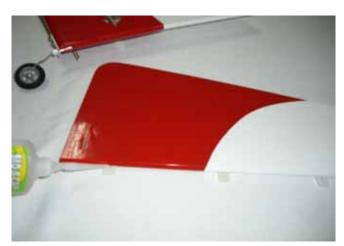
$\square$  step 7 Carefully put some drops of medium CA into the 2 mm hole into the rudder. Carefully locate the rudder and glue the hinges with some drops of thin CA.
