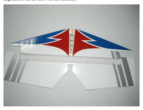
$\Box$  step 2 Carefully glue the hinges, with some drops of thin CA, in the elevator only. Than insert carefully the elevator through the fuselage.
