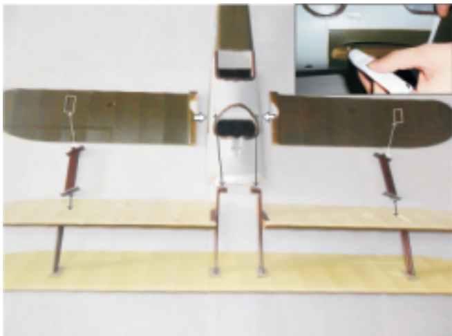
5. coated Mucilage at the third wing and another support frame junction.
