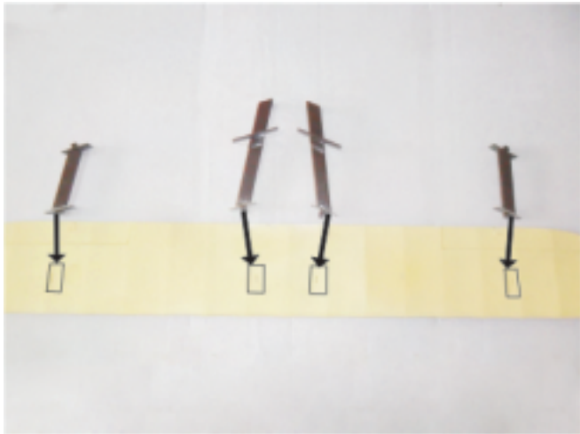
1. Coated Mucilage at the top wing and support frame junction.
