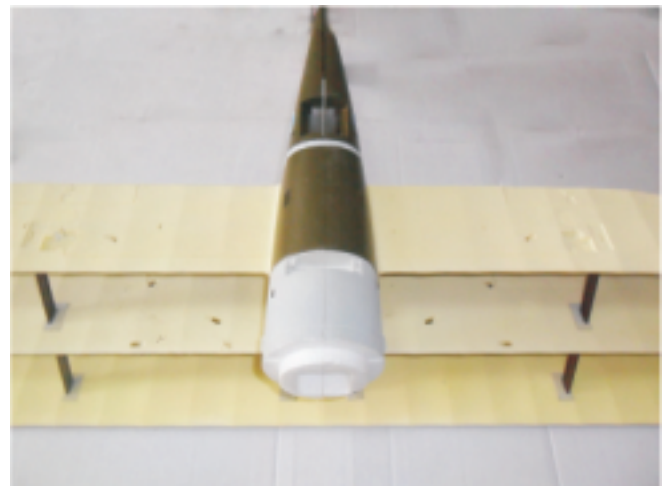
6. Stick the support frame on the third wing junction.
