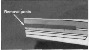
□ 6. Located at the rear of the fuselage, behind the horizontal stabilizer slot, are the balsa tail posts. These posts were left for manufacturing alignment. The posts must be removed in order to insert the horizontal stabilizer. Using a sharp hobby knife or razor saw, cut the posts even with the slot as shown in the picture.
