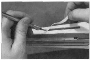
□ 7. Using your finger, locate the vertical fin slot on the top of the fuselage. Remove the covering with a hobby knife.
