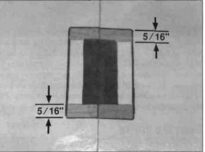
□ 13. Hold the plywood aileron servo tray over the hole in the bottom of the wing. Trace the outside of the tray with a felt tip pen and then remove the tray from the wing. Draw two lines 5/16" from the ends as shown. Carefully remove only the covering within the lines using a new #11 blade in a hobby knife, being careful not to cut into the balsa wing sheeting.
