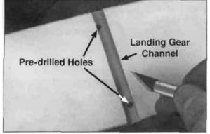
□ 24. On the bottom of the fuselage, there is a channel for the main landing gear. Locate this channel by running your finger over the covering on the bottom of the fuselage. Using a hobby knife, remove the covering from this channel.
