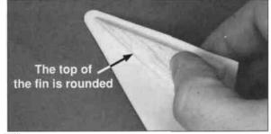
$\Box$  16. Attach the white decal to the balsa dorsal fin by wrapping it around the top. Trim off the excess decal material even with the edges. Do not apply to the flat bottom or aft edges
