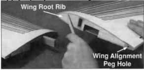
□ 11. Apply epoxy inside the joiner cavity of the remaining wing panel. Next, coat the wing root ribs on both panels. Insert the wing alignment peg into the hole at the trailing edge. Quickly proceed to the next step.
