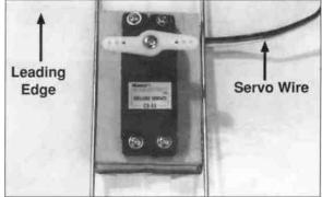
$\Box$  58. Install the remaining servo into the servo mount in the wing. Route the wires between the tray and the bottom of the wing as shown.
