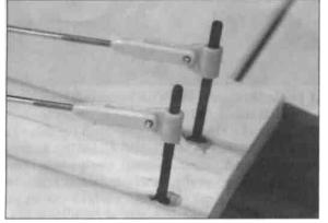
**22.** Attach the pushrods to the aileron control horns. Press the forks of the clevis together until they snap into place.
