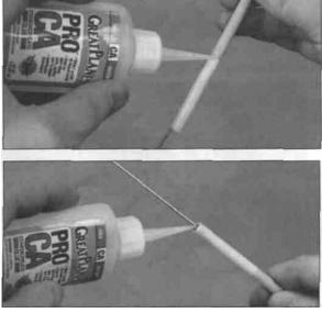
□ 61. Locate the two wooden dowel pushrods and apply thin CA to the ends of the shrink tubing on both rods.
