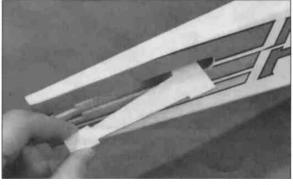
□ 4. Locate the 1/8" (3mm) plywood stabilizer mounting base and trial fit it into the bottom of the horizontal stabilizer slot. Lightly sand the base if necessary to obtain a good fit. Remove the base from the fuselage.
