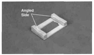
□ 15. Glue the balsa aileron servo blocks onto the servo tray so that the angled side you just cut is facing away from the plywood tray.
