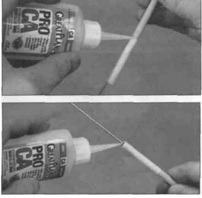
□ 61. Locate the two wooden dowel pushrods and apply thin CA to the ends of the shrink tubing on **both rods.**
