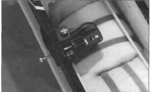
□ 60. Cut out the opening on the left side of the fuselage for the switch and install using the screws included with the switch. We recommend using a GreatPlanesSwitch/Chargelack(GPMM1000,shown above.) This makes it easy and convenient for charging your receiver batteries. It is good practice to always install the switch on the side opposite the engine's exhaust.
