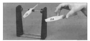
We use a Top Flite Precision Magnetic Prop Balancer (#TOPQ5700) in the workshop and keep a Great Planes Fingertip Balancer (#GPMQ5000) in our flight box.
