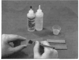
□ 2. Mix approximately 1/4 oz. (7.5ml) of 30-minute epoxy using a mixing stick and a cup. Using a mixing stick or epoxy brush, apply an even coat of epoxy on
