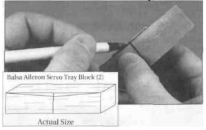
□ 5. After the epoxy has cured and the clothespins have been removed, draw a centerline on both sides of the plywood wing joiners and the two balsa 5/16" square x 1-7/16" (8mm square x 36mm) aileron servo tray mounting blocks. Use the plywood joiner as a template to mark the wing dihedral angle on both of the balsa aileron servo tray mounting blocks. Put the balsa blocks aside for use in later steps.
