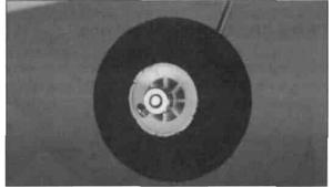
$\Box$  77. Place one wheel collar on each strut, followed by a wheel. Secure each wheel with an additional wheel collar. The wheels must all spin freely and have no tendency to bind.
