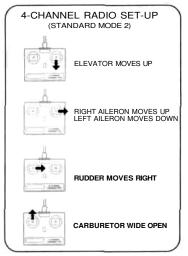
If any of the servo movements are opposite, reverse the servo direction with the servo reversing switches on the transmitter.
