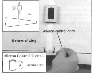
**Q** 20. Thread (he aileron control horns onto the torque rods until there is 3/4" (19mm) of torque rod between the wing and control horns.
