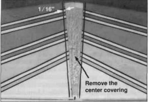
$\square$  13. Remove the stabilizer and draw two additional lines, on the top and bottom, 1/16" inside the lines
