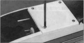
□ 45. Place the hatch onto the fuselage and drill 1/16" holes, using the holes in the hatch as a guide, through the hatch and into the mounting blocks. Fasten the hatch using the four 2 x 12mm flanged sheet metal screws.
