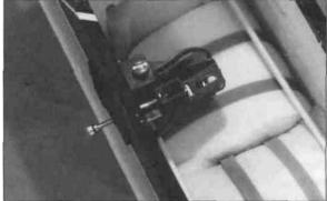
□ 60. Cut out the opening on the left side of the fuselage for the switch and install using the screws included with the switch. We recommend using a GreatPlanesSwitch/Chargejack(GPMM1000, shown above.) This makes it easy and convenient for charging your receiver batteries. It is good practice to always install the switch on the side opposite the engine's exhaust.
