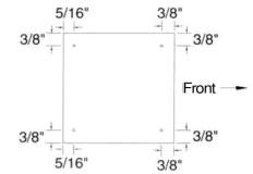
$\Box$  44. Drill four 1/16" holes into the tank hatch as shown in the sketch.
