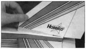
□ 15. Trial fit the fin into the slot in the top of the fuselage. Sand the edges if necessary for a snug fit. Mix 1/4oz. (7.5ml) of 30-minute epoxy. Using a mixing stick, apply epoxy to the top of the horizontal stabilizer through the slot. Apply epoxy to the sides and bottom surfaces of the fin base that have balsa wood exposed. Insert the Fin into the slot, making sure the fin base is seated firmly on the horizontal stabilizer. Check for a perpendicular angle between
