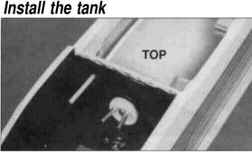
$\Box$  43. With the vent tube (inside the tank) pointing up, insert the fuel tank into the fuselage. Make sure the foam collar is seated well against the firewall.
