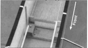
$\Box$  55. Position the servo tray support into the fuselage directly in front of the the landing gear block. Glue in place with thick CA.
