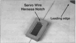
$\square$  17. Mix l/8oz. (3.5ml) of 6-minute epoxy to glue the servo tray to the bottom side of the wing. Apply
