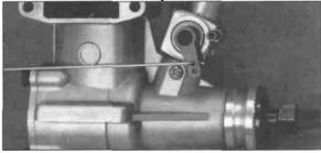
**49.** Attach the "Z" bend of the remaining 1/16" x 18" wire pushrod into the inside hole of the carburetor control arm.
