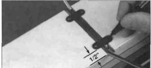
□ 26. Position the two wire struts in the holes inside the channel. Center the two landing gear straps over the struts so they are approximately 1/2" from the sides of the fuselage. Mark the holes using a felt tip pen.
