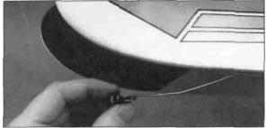
□ 35. Attach the "Z" bend ofOne of the wires into the outside hole of the black plastic steering arm. Slide the wire into the plastic guide tube so that the screw hole on the steering arm is facing forward. Slightly bend the wire as needed so the arm can be positioned close to the nose gear mount (see photo at step 36).
