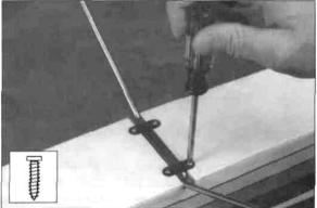
$\square$  28. Using four 2.5 x 10mm self-tapping screws, fasten the landing gear straps to the bottom of the fuselage over the struts.
