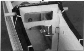
■ 29. Cut a small notch that is 1/8" wide and 1/8" deep into the front fuselage former approximately 3/4" down from the top of the fuel tank opening. This will give the throttle pushrod a straighter line to the servo. Cut the two white plastic pushrod guide tubes **so** they are both 11" long.
