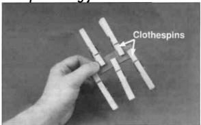
**4**. Use clothespins to clamp the wing joiners firmly together. If any more epoxy squeezes out, remove using a paper towel. Make sure the joiners are evenly lined up with each other, set this aside until fully cured.
