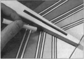
□ 12. With the stabilizer properly aligned, using a felt tip pen, trace a line around the tail of the airplane on the top and bottom of the horizontal stabilizer.
