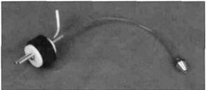
$\Box$  40. Locate the metal fuel pick-up weight (often referred to as the "clunk") and the fuel tubing. Cut the fuel tubing so it is only 5-1/2" long. Attach the fuel tubing to the short aluminum tube and to the clunk.
