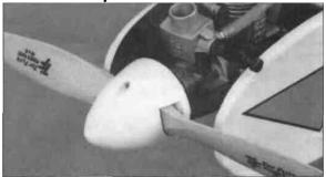
□ 53. Trim the spinner cone slots if necessary so there is at least a 1/16" gap between the cone and the prop. Once satisfied with the fit, attach the cone with the screws provided. Be careful not to over-tighten these screws. They are threaded into plastic which can strip out easily if they are over-tightened.
