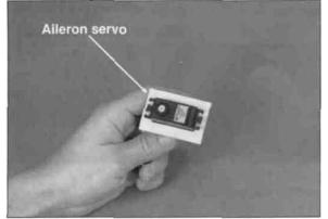
□ 16. Trial fit the aileron servo into the servo tray and the hole in the bottom of the wing. Enlarge either hole, if needed, with a hobby knife or a fine-toothed file until a proper fit is achieved. The plywood tray should not actually contact the servo. Leave a 1/64" gap all the way around. Remove the servo.
