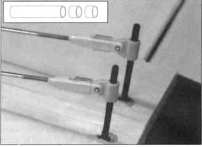
□ 23. Locate the 1/4" (6.5 mm) diameter clear retaining tube and cut two 1/4" (6.5 mm) pieces. Slide one piece onto each clevis to secure the connection between the clevis and the horn.
