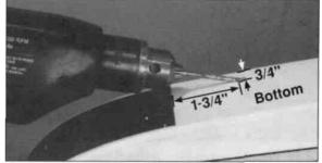
□ 31. Measure and mark the steering pushrod exit onto the **bottom** of the fuselage 1-3/4" back from the fuselage and 3/4" in from the left side as shown. Using a 1/8" drill bit, drill a hole that angles in towards the back of the fuselage as shown. Be careful not to let the drill chuck damage the covering.
