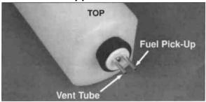
□41. The stopper assembly can now be inserted into the tank. The pressure tube should be adjusted so the tube is pointed straight up just under the top of the tank. The rubber stopper must seat over the lip of the tank. Make sure that the tubes are positioned side-toside. Tighten the stopper by turning the screw. Do not over-tighten or you may strip out the plastic disk.
