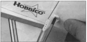
□ 20. Drill two 3/32" (2.4 mm) holes straight through the balsa rudder at the marks. Place a drop of thin CA into each hole. This will add strength to the balsa. Redrill the holes to remove any excess glue. Insert two 2 x 20mm machine screws through the control horn, and rudder, then finally screwing them into the control horn back plate on the opposite side of the rudder. Tighten the screws but do not crush the balsa. Cut off the excess threads that stick out using a wire cutter.
