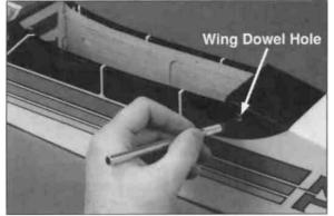
□ 1. Locate the four round holes, two on each side of the fuselage, and remove the covering over each hole. Caution: Do not cut out the rectangular holes in the side of the fuselage.
