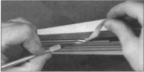
□ 3. Locate the horizontal stabilizer slot under the covering on the tail section of the fuselage by pressing lightly with your finger. The slot is located on both sides of the tail. Using a hobby knife, carefully remove the covering, exposing the slots. NOTE: Do not cut into the wood around the slot.
