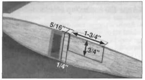
□ 7. Mark the aileron servo location on both wing panels using a felt tip pen. Using a hobby knife, cut an opening into the panels following the lines you just drew.
