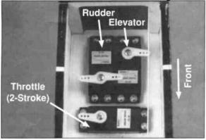
□ 57. Routing the servo wires forward, install the servos into the tray as shown using the screws included with the radio system. Enlarge the openings if needed.
