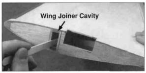
□ 10. Mix 1/2oz. (15ml) of 30-minute epoxy. Use a mixing stick or epoxy brush to apply epoxy to all four sides of the joiner cavity wall. Insert the joiner into the cavity up to the centerline marked on the joiner plate. Be sure you are installing the joiner correctly. Quickly proceed to the next step.
