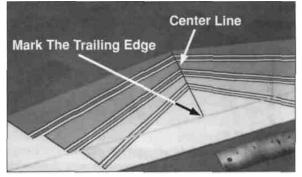
□ 9. On the top surface of the **horizontal stabilizer**, measure to find the exact center from side to side. Draw a "center line" using a felt-tip pen. Next, extend that line onto the trailing edge, in the hinge gap, as shown. (DO NOT MARK ON THE ELEVATOR.)
