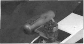
□ 51. Install the muffler onto the engine using the screws that came with the engine. Attach the fuel tubing from the "vent" in the fuel tank to the muffler pressure tap. Attach the tubing from the fuel tank to the carburetor. NOTE: You may wish to shorten the fuel lines for a more direct routing. Make sure that the lines do not get any kinks which could restrict fuel flow.
