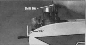
□ 46. Position the engine on the mount so that the face of the engine thrust washer is 1/4" forward of the fuselage sides. Align the engine so the crankshaft is pointing straight forward. Mark the rails at the four mounting holes using a 5/32" drill bit (or a bit that fits your engine mounting holes the best) to scribe a mark. Note: You may need to trim the mounting rails slightly to fit your engine—this can be done with a flat file.
