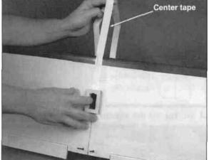
$\square$  18. Starting at the front of the aileron servo tray, apply the 1/2" (12.5mm) white wing center tape completely around the wing over the joint. A small amount of pressure should be applied to make a smooth seam.
