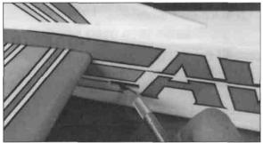
□ 23. The pre-cut elevator pushrod exit hole is located on the same side of the fuselage as the elevator control horn. Locate the exit hole by gently running your finger along the side of the fuselage over the covering. It should be located approximately 1/2" in front of the stabilizer where shown. Using a hobby knife, remove the covering from the elevator pushrod exit hole.
