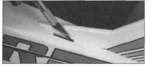
$\square$  22. The pre-cut rudder pushrod exit hole is located on top of the fuselage on the same side as the rudder control horn. Using a hobby knife, remove the covering from the rudder pushrod exit hole.
