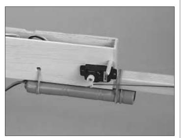
□ 3. After the plane is properly balanced, mark the location for the motor battery. The motor battery is held on to the fuse with two small rubber bands. Our plane balanced with the motor battery mounted under the two servos. We attached the aft end of the battery to the fuse with a small rubber band. Make a small hole through the wing pylon and route a second small rubber band through the hole and attach it to the front of the motor battery.
