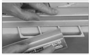
An easy method to hold the delicate tail pieces while sanding the edges is to place the edge of the tail piece over the end of your building table. Position a second sanding bar on top of the tail piece, approximately 1" (25.4mm) back from the edge. The tail piece can now be held evenly and securely by applying slight pressure on the sanding bar.
