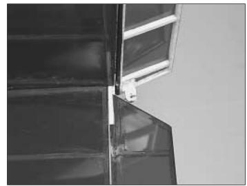
□ 6. Glue the die-cut 1/16" (1.6mm) plywood **rudder** and **elevator horns** in the slots in the rudder and elevator. **Note:** Use a pin to enlarge the holes for the pushrods, if needed.
