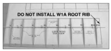
□ □ 5. Starting at the wing tip, glue the seven laser-cut 1/16" (1.6mm) balsa W1 and one W1A rib over the main spar and trailing edge sheet, perpendicular to the building board. Important: Do not install the W1A root rib until the next step.
