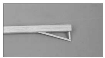
□ 15. From a 1/8" x 1/8" x 24" (3.2mm x 3.2mm x 609.6mm) balsa stick, assemble a tail skid and glue it to the bottom aft end of the fuselage.
