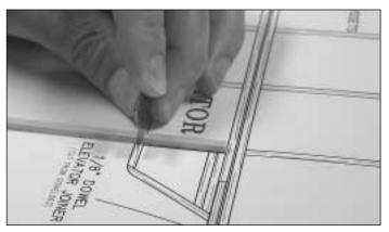
1. The easiest way to cut balsa sticks is with a single-edge razor blade. To do so, position the stick over the plan, then place the razor blade on the stick where you wish to cut it. Press down lightly on the razor blade to make a mark where the stick is to be cut.
