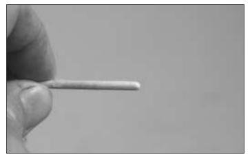
□ 1. From the remaining 1/8" (3.2mm) hardwood dowel cut two **wing hold downs** 2" (50.8mm) long. Use a sanding bar to round the ends of the wing hold downs.
