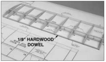
$\Box$   $\Box$  8. Cut one of the 1/8" x 24" (3.2mm x 609.6mm) hardwood dowels so that it fits in the notches at the front of the wing ribs, from the root to the tip rib. Glue the dowel to the ribs. Save the excess dowel for use as a wing hold down dowel.
