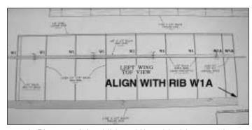
□ □ 4. Pin one of the  $1/32" \times 3/4" \times 24"$  (.8mm x 19mm x 609.6mm) balsa **trailing edge sheets** in position over the plan, aligning one end of the trailing edge sheet with the outside edge of the root rib W1A.
