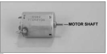
□ 1. Use denatured alcohol or other solvent to clean the motor shaft. Roughen the shaft with 320-grit sandpaper so glue will adhere.
