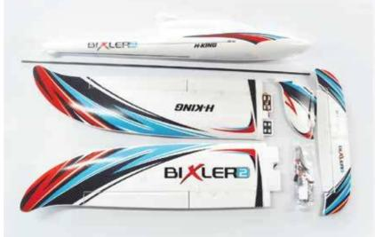
place by fixing the screws thru the bottom of the fuselage. When you need to remove the wings from the fuselage, use a philips screw driver to unscrew it and also pull the wire as shown at the same time to take the screws out from the access hole.
