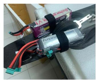
the main fuselage below the nose gear tray and then fixed with 1-2 small velcro loops (not cable ties) to the board, which allows you to quickly unhook the wires and take the nose gear board off. Of course you have to be careful that the nose gear cannot get tangled in the battery wires.
