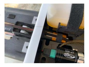
Make sure that the motor of the gear unit fits through the front face of the main fuselage and clears the RC equipment board inside. There should be a few mm clearance around the motor, that under no circumstances this motor could be hit or bent. As you see, you can slide the nose dual carbon tube unit in and out easily and just secure it with two M4 bolts through the aluminum angle brackets.
