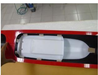
Then, when the glue has set, install the vacuum formed cockpit from inside, of course after you painted it to your liking. If you have a few instruments or side panels lying around, they would for sure enhance the looks of the cockpit. We have decided that the CARF-Models BOLT! looks too good to not boast a clear canopy and a cockpit, so that little extra work is well invested and you will love the result. use 6-8 scrap balsa blocks and a thin plywood in the front to secure it removable.
