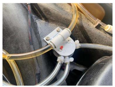
also take care that the smoke injector tube clears the canopy hatch when sliding it back into position on the main fuselage, and that it isn't in the way when removing the bypass cover to quickly access the engine. A bit tricky, but it can be done and it is the best way to do it.
