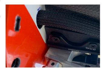
Now grind an opening in the vertical surface of the removable nose part exactly where the connector is to be placed. Then slide the female part on the connector in the fuselage, apply a little 5 min epoxy on it and slide the nose hatch over it. Wait 10 min until the 5 min Epoxy has set and then pull the nose off. Now you can crate a nice fillet around the connector in order to have a very safe connection for the nose gear servo.
