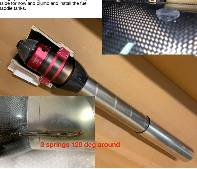
**Fuel tanks:** Plumb the saddle tanks now. We only use 2 lines (one in, one out). The out line is the clunk line. Put a brass tube in the baffle area so that the baffle cannot damage the fuel line. The in-line will be bent so that the tube reaches the top corner of the fuel tank.
