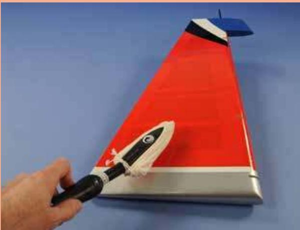
2) Using your covering iron with a soft sock, gently apply pressure and rub in the covering. If any bubbles occur, your iron may be too hot. Reduce heat and work slowly.
