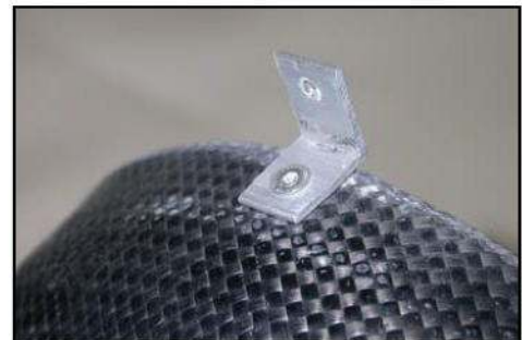
(bottom) Bellmouth brackets secured to F6 with small screws.
