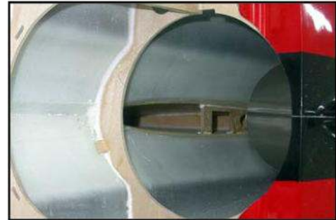
(above) Rudder servo mount is installed for you at the factory. (below) Servo installed with balsa protection glued in position.
