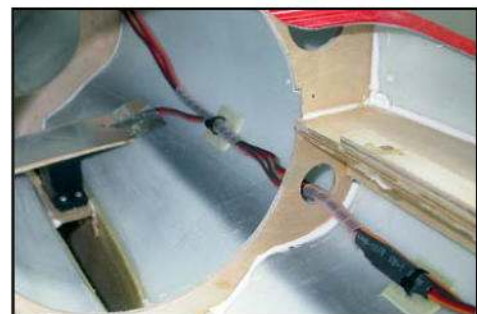
(above) Secure rudder & stab servo extensions to fuselage. Cover rudder servo plate with aluminium tape for heat protection. (below) Rudder linkage fairing.
