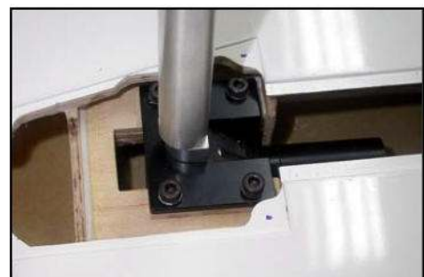
(below) Retract installed on the wing mount. Trim around cutout in wing as needed, and keep aligned with wheel-well.
