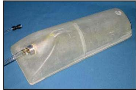
(above) The fuselage tank completed, ready for installation.
