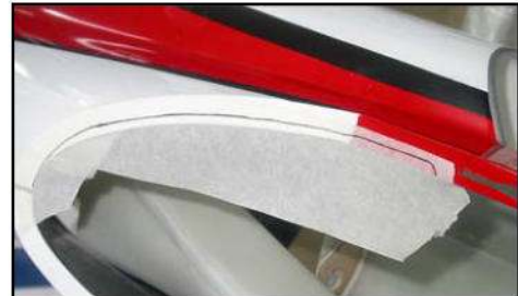
(below) Trim the flanges of the cockpit area as shown to fit the the fuel tank.
