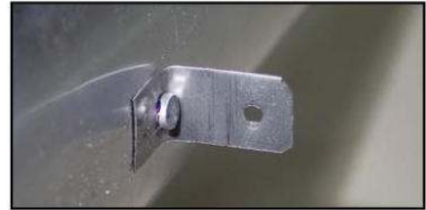
(above) Drill \varnothing 3mm hole in brackets on outer tube.
