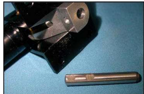
(above) You must grind small 'flat's on all the connecting pins and axles when assembling the Landing Gear. Use a drop of loctite on all set-screws for safety
