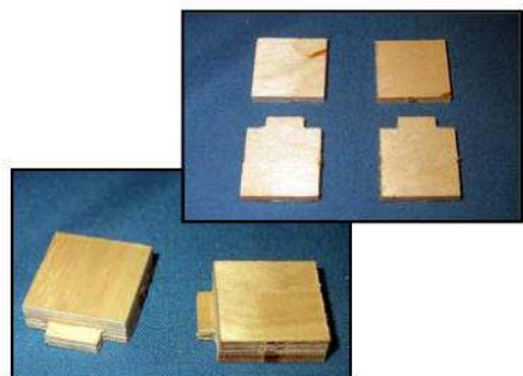
(above & below) Upper bypass ducting is secured to these 2 blocks with M3 bolts & T-nuts.
