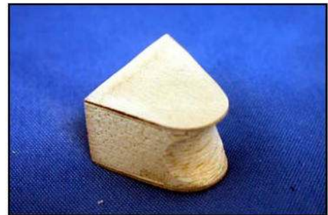
(above) Block is made from sandwich of 0.8mm plywood and 10mm balsa. Shape as shown. (below) Adjust thickness of block and depth of radius so that door just clears oleo knuckle when opening, and closes completely.
