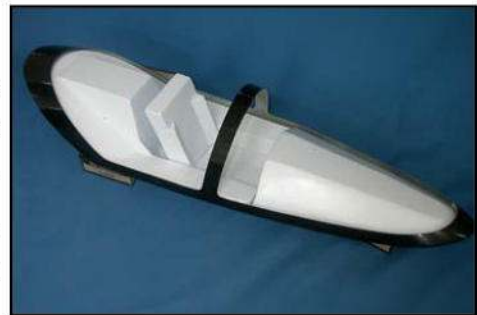
(below) Plastic cockpit tub dry-fitted into the cockpit. Add detailing and paint as required.
