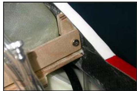
(below) Front stop is a milled plywood strip, screwed to small milled blocks glued against the fuselage sides.
