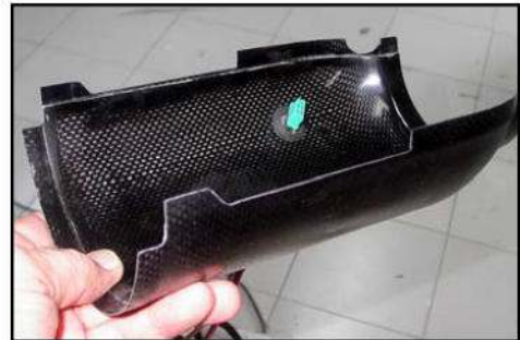
(below) Bypass cover trimmed ready for final installation.
