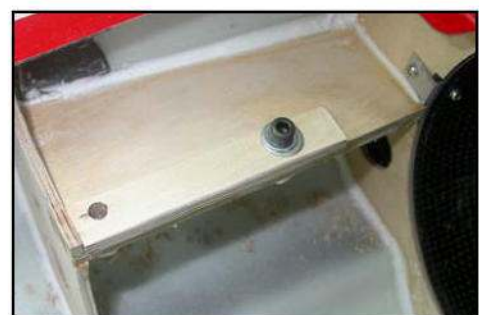
(above) Glue spacers onto the factory-installed engine mounting rails to centre your turbine in the bypass as necessary.
