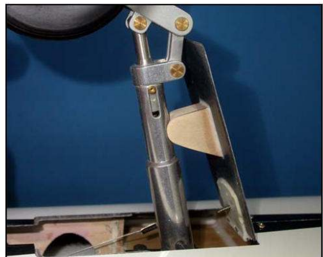
(above) Block is made from sandwich of 0.8mm plywood and 10mm balsa. Shape as shown. (below) Adjust thickness of block and depth of radius so that door just clears oleo knuckle when opening, and closes completely.
