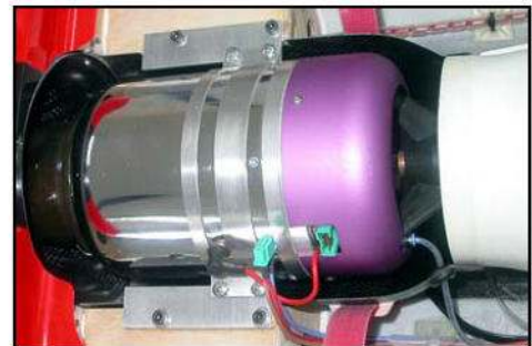
(above) Inlet ducts are factory-installed and painted for you. (below) General view of P120 installed in carbon bypass duct.
