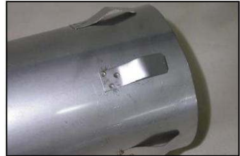
(below) Bend the 6 tabs at back of inner tube into 'V' shape.
