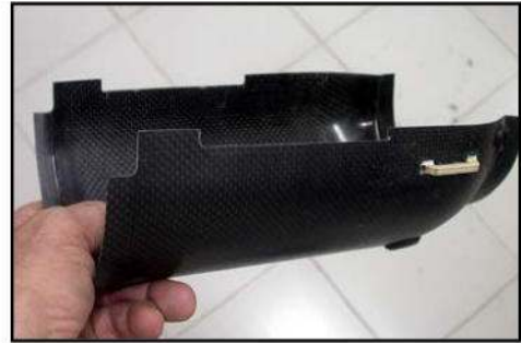
(above) Upper bypass trimmed for P80/P120 installation.
