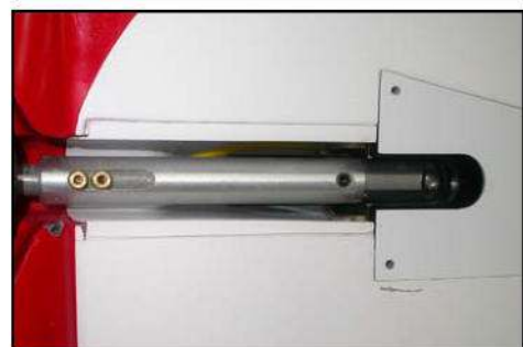
(above) Mark the slots on the servo covers exactly in line with the oleo legs, and mill as shown. Make them at least 38mm long, so that there is space for the brake tube to enter the wing outboard of the retract unit.
