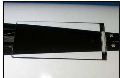
(above) Nosegear door hinge glued and screwed in position. (below) Nose door should have 1mm gap all round.
