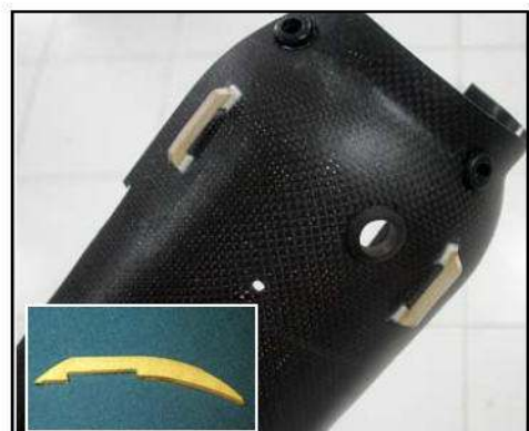
(below) View of upper bypass, showing plastic grommets for tube and cable protection and hoops to retain Velcro strap. Inset is CNC milled hoop included in kits
