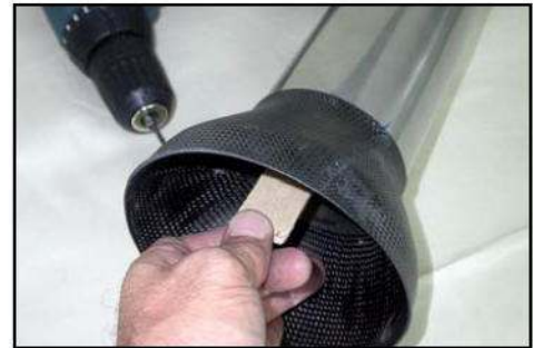
(above) Fix carbon bellmouth to inner tube with rivets or screws.
