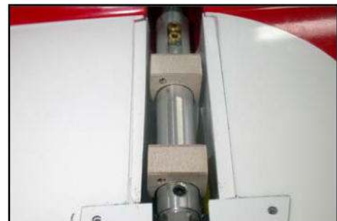
(above) The blocks to support the gear doors are 10mm balsa strip and 0.8mm ply sandwich. Shape with a Dremel sanding drum. (below) The blocks are glued to oleo legs with CA.
