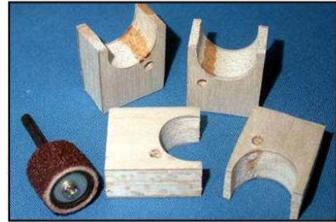
(above) The blocks to support the gear doors are 10mm balsa strip and 0.8mm ply sandwich. Shape with a Dremel sanding drum. (below) The blocks are glued to oleo legs with CA.
