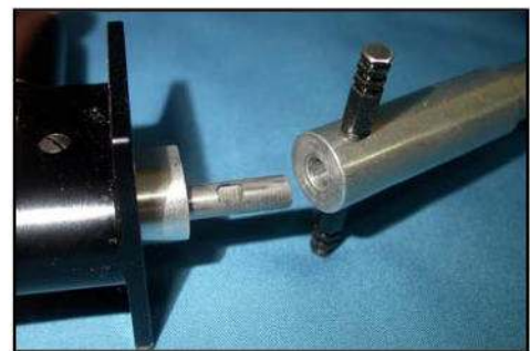
(bottom) Nosewheel oleo with axle and centering tubes.
