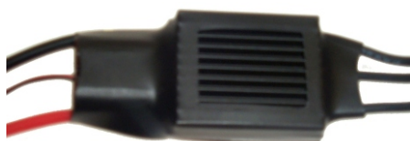
Recommended West 770KV motor and 60A controller, 4 cell 3350 lipo. (Up to 15mins flying time)
