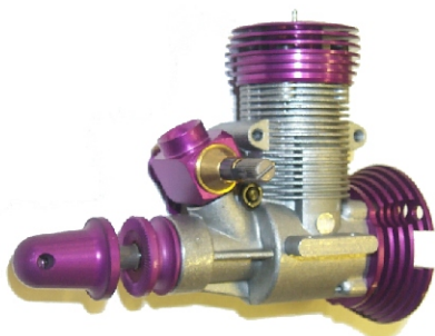
Recommended motor West 36TIR and Genesis pipe. (Which produces over 2.2BHP)
