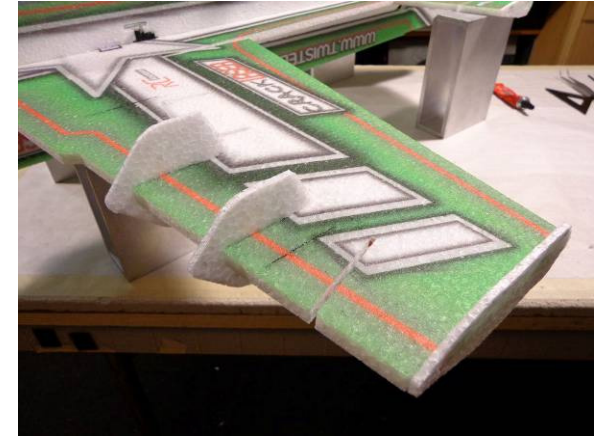
Attach the three different SFGs to each wing as shown... Welders or CA can be used to install these
