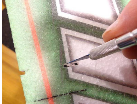
Clean out the slots on the wing for the SFGs, test fit them before applying the glue.
