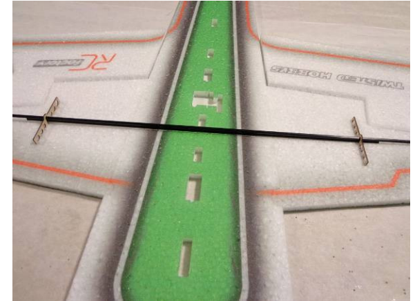
Gently lower the spar/rib assembly into its precut area. Notice that the shorter center spar should be centered and entering the wing first
