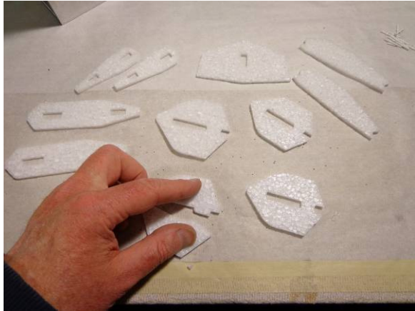
Cut all the shown parts from there EPP foam trees, split the rear of the 4 inboard SFGs as shown
