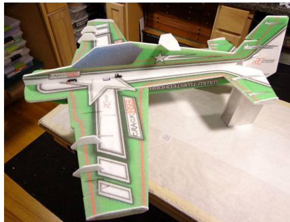
Lastly the T-Canalizer. Make sure all the add-ons are all perpendicular to their respective surfaces
