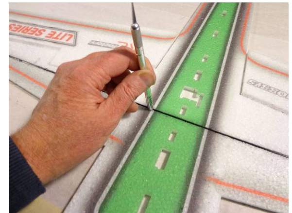
Lower the spar/rib assy back into the wing like was done on the dry fit. Press down in all areas to fully seat the spars and ribs into their respective slots
