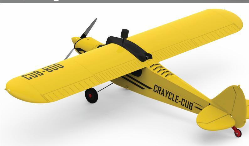
You can also prefer the Hatch1\_flat and Hatch2\_flat to make to model real scale if you fly without FPV. Use 2 mm screws to mount Hatch2 and drill before screwing.
