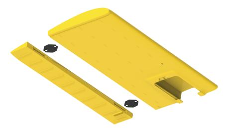
Take the servo as position as the same in the image below and screw onto the "wing1" part. Then you can glue the "wing1""wing2" and "wing3" parts together. Be careful not to apply glue to the servo and same process goes for the other side.
