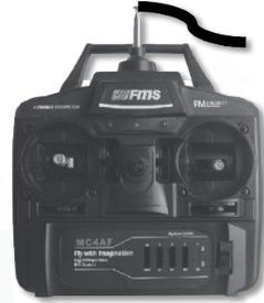
2. Attach a small wind ribbon to your remote control's antenna and fully extend the antenna - not necessary with 2.4 GHz transmitters.
