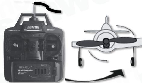
5. Press the throttle control on your remote control briefly and carefully and the air-screw will start rotating.
