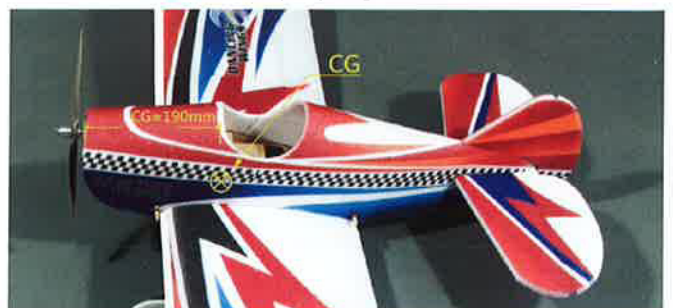
0.18 Assemble the battery, receiver, and adjust the C.G, now you could try flying.
