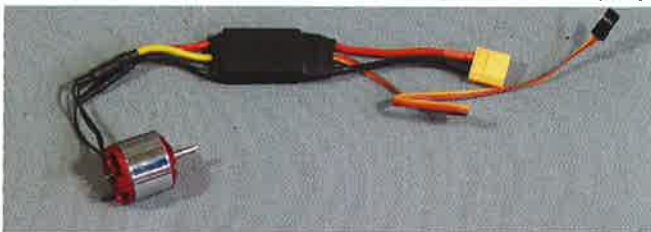
0.14 Connect the motor and ESC together, assemble the motor on the fuselage and fix with screws (U1).
