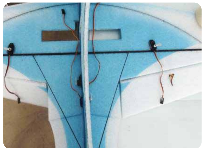
14. Install elevator and rudder servos onto the fuselage as shown. From the bottom view, left is the elevator servo and right is the rudder servo.
