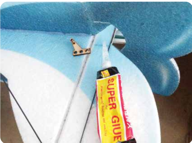
11. Assemble quick rod adjusters to the plywood control horns.
