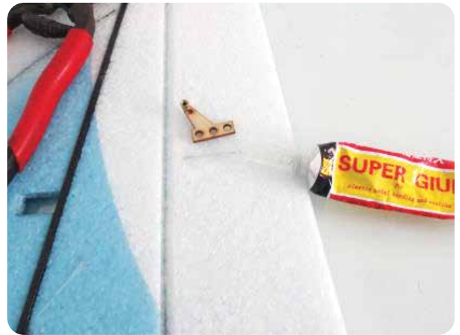
12. Apply glue and install all the control horns to the control surfaces as shown.
