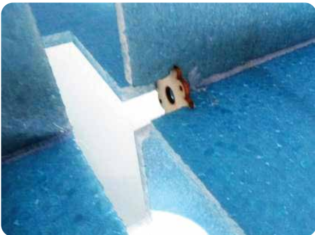
19. Hot glue the motor mount onto the fuselage.
