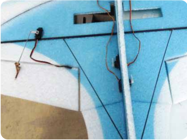
16. Install push rods onto the control horns, hook up to the rod adjuster and tighten the grub screw when the control surfaces are perfectly levelled.
