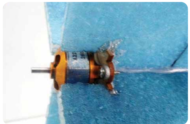
20. Install a motor mount on the plywood mount.
