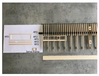
The next step is the border for the flaps in the wing. The parts KF1-KF2 from the 3mm, and the two strips KF3 from the 2mm balsa board are needed. KF3 can be found on the balsa board of the ribs (part A). Note here that there are two different versions of KF3: one with the cutout for a servo frame, and one without the cutout. The parts are inserted into the surface in the recesses provided for this purpose and glued. The short KF2 strips are always glued to
