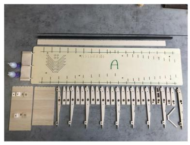
**Tip:** take enough time with such a large number of ribs to align them neatly with the combs on the base plate. The end ribs A25 must again be inclined 5 degrees with the template. The gap between the two ribs A1 in the center is larger than the gap of the remaining ribs. As a result, the comb does not fit into this gap either. In order to align the ribs at a 90 degree angle to each other, we clamp the relining to the surface screw A2V (8mm balsa board) between
