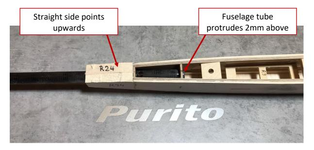
The final work on the hull now includes the transition from the hull boat to the hull tube, which is done with the two parts R24. These are fitted to the end of the fuselage boat and glued with the straight side facing upwards.
