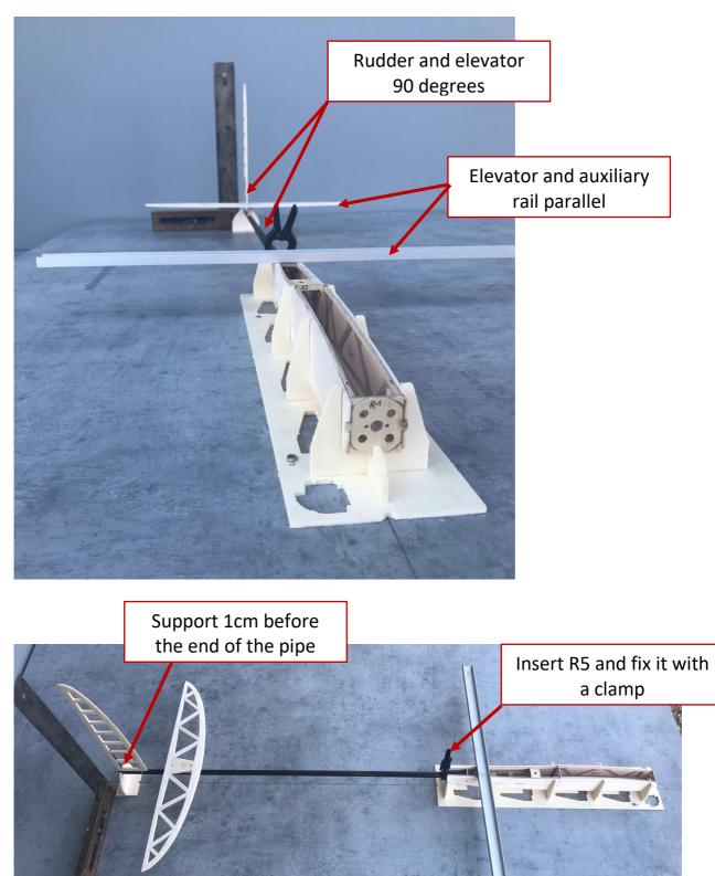
A straight line is drawn on the building board, extending along the entire length of the hull. The fuselage tube is inserted into the fuselage boat so far that it protrudes 2mm from frame R4.
