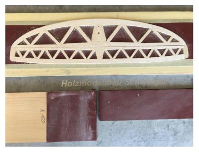
Tip for sanding the tail unit: We stick a piece of sandpaper over the entire length of the tail unit on a wooden plate. The tail unit is placed on top of this, as can be seen in the picture.
