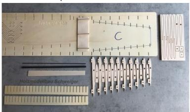
On the picture you can see the needed parts: Base plate, matching ribs for part C, edge bow, 5 degree stop, end bar, comb, 7mm CFK tube (spar) and the 2mm CFK tube (leading edge).
