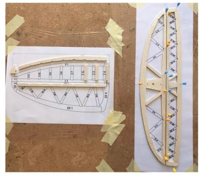
The 4mm balsa board with the parts for the elevator and rudder are needed for building. The reinforcement part made of 4mm poplar plywood is in the accessories package. Additionally there are 3 parts (S4-S6) for the rudder on the 8mm balsa board.
