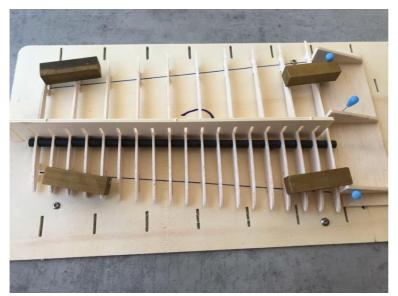
One more note about the base plate: The foot at the end strip of the rib determines the position.
