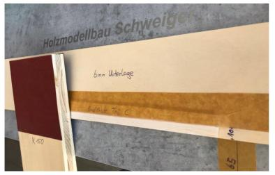
The end strips are ground before installation. To do this, place the first and last ribs on the end strip and mark the end of the ribs on it.
