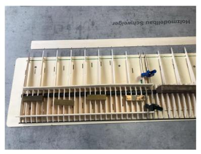
After that, the two plywood pieces A1V (for the surface screw connection) can be placed. These belong in the recess of the plywood ribs A1. The top side is marked by the recess for the screw head.
