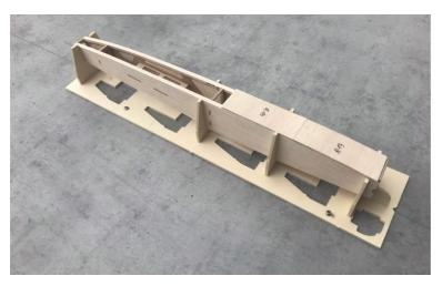
Now the hull boat can be taken out of the slipway and inserted with the bottom side facing upwards.
