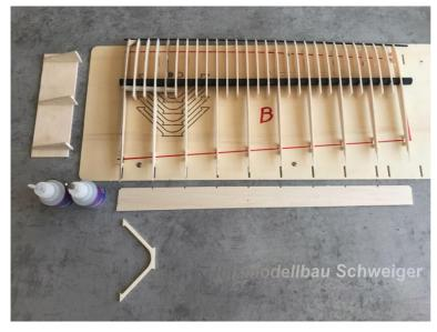
The wing panels B are built up in the same way as the wing panels C.
