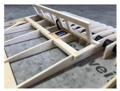
Should our solution be used for the flap opening, a servo arm extension is required. For the servo arms we recommend our GFK extension, which is available as an accessory together with the matching servo frames.. We also have a video for the functional mode: https://youtu.be/d9o5HwRrMTI
