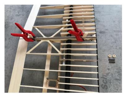
To prevent twisting of the wing ears on the center section, the accessory package includes dowel pins with a diameter of 2.5mm made of CFK. These pieces are slightly sharpened with sandpaper and inserted into the wing center part. Now the ear can also be pinned on, but with a small gap to the root rib.
