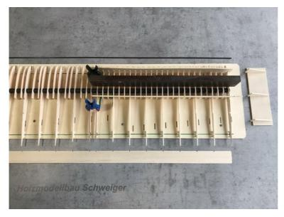
Now the remaining ribs can also be aligned. They are then glued to the spar. After this step, the leading edge (CFRP tube 2.5mm) can be attached to the front. Note that the comb must be shortened by one field to align the ribs. This is because the root rib is now at an angle of 5 degrees and thus the comb no longer fits over a complete half of the center section.
