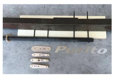
The pylon part P1 can now be fitted and glued in place. For component P2, make sure that the M3 nut points downwards. Attach and glue the P2 and P3 components as well. Only part P4 must not be glued yet, because this will be done later with the elevator. The carbon rods that protrude from the top of the elevator pylon should be shortened to 4.5mm (so that they no longer protrude when the elevator is screwed on)
