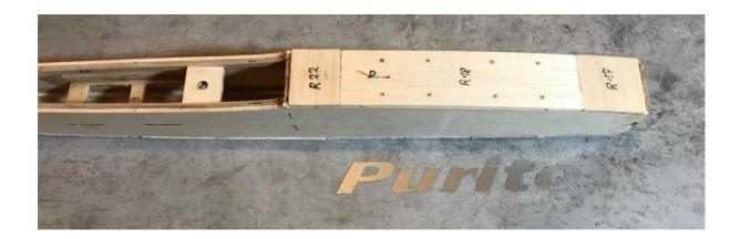
The plywood part R23 is glued inside the canopy to the fuselage tip center, serving as a tongue. Glue the balsa part R21 to the end of the canopy between the plywood strips. Bend a steel wire into L-shape and glue it together into a Bowden cable into the inside of the canopy as a fastener.
