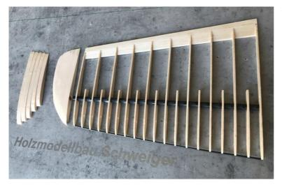
The parts for the edge bow (1-5) can be found in the 8mm balsa board. These can be glued together according to personal taste, we use an offset at the end strip of about 2mm. Tip: protect the building board here with a piece of household foil, place the parts of the edge bow with the straight underside and glue them together.
