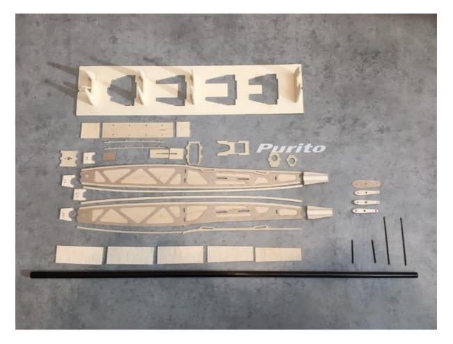
On the 2nd picture you can see all the parts that are needed for the construction. The parts are arranged in the picture as they will be assembled. The 0.6mm plywood reinforcement R10 is already glued to the balsa side R9 with white glue. The right half of the fuselage is the shorter side, so parts R7 and R8 are also shorter. They are glued together with R6 to the fuselage half as shown in the picture.
