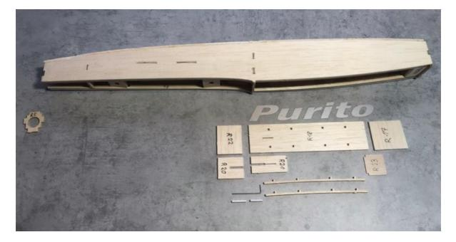
**Be careful here:** part R17 is again beveled on one side due to the engine side pull. Glue the two symmetrical plywood parts R19 into the canopy R18 in the holes provided. Make sure that the canopy reaches the necessary bend.
