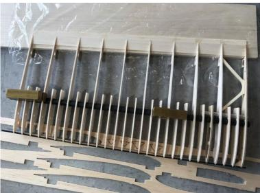
The wing part B is again underlaid at the leading edge with 2mm (under the feet of the ribs) and at the trailing edge with 8mm. This allows the end strip to be glued on without distortion. At the end, the large reinforcement between rib B1 and B4 is glued in place. The reinforcements are made of 3mm poplar plywood. These reinforcements will help us later to string the wing without distortion.
