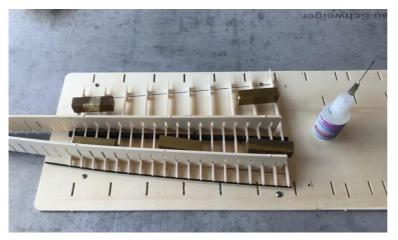
At the end we check again the correct alignment of all ribs and glue all whole ribs (not the halfribs) to the tube. Tip: for correct alignment we use weights to fix the wing part neatly. We use a thin liquid super glue for gluing. For the leading edge we use the 2mm CFK tube, which is carefully inserted into the cutouts provided for it.
