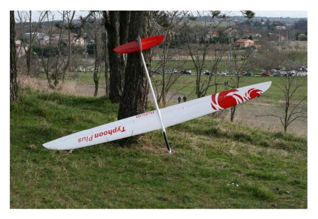
TYPHOON Plus is the big brother of the typhoon 2m. with a wingspan of 2m90, it's a f3f glider. The quality of construction allows it to fly ballast and go fast without any problem. You have as much fun to fly this version of the typhoon thanks to its maneuverability and kindness in flight.
