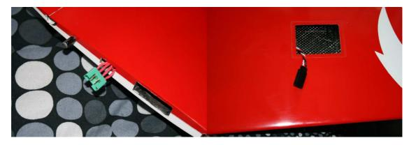
Before installing the servos, put in neutral for the aileron servos. Provide an offset of 20 ° for the flap servos. This is to be a large movement of the flaps.
