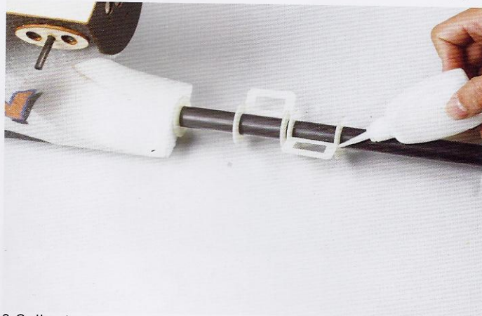
3. Splice two sets servo mounts .
