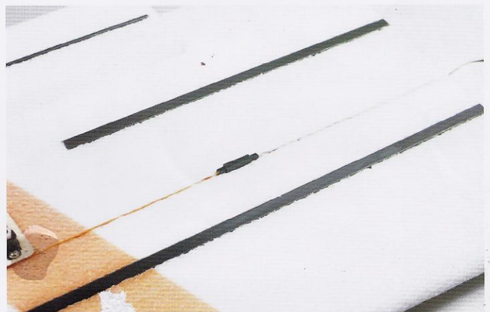
9. As you see in the picture, please embed the servo wire and extension line into the foam.
