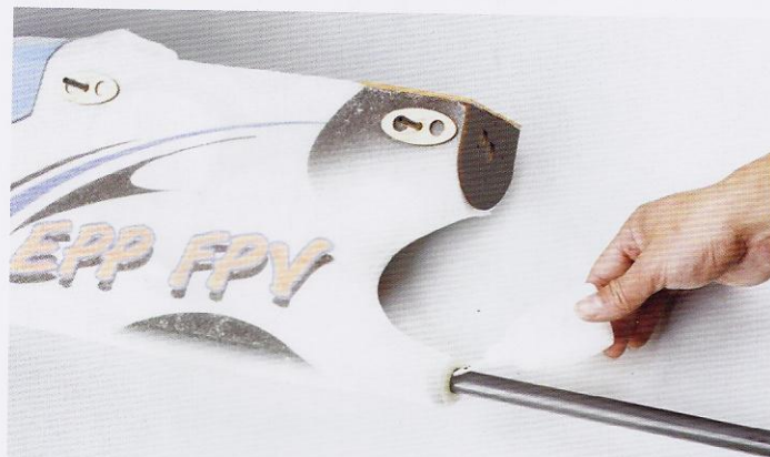
1. Splice rubber band bolt 2pcs diameter.5mm*130mm(L)
