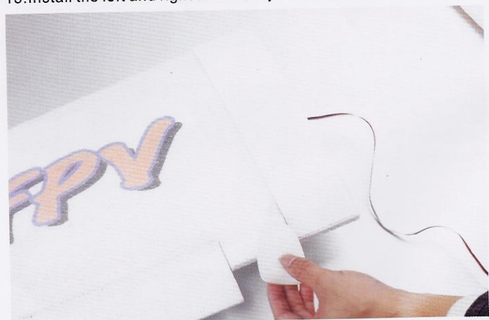
16. Splice Abs board to left and right wings . 2pcs
