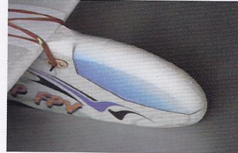
33. Install the battery. Attention: please adjust the plane's key point position.
