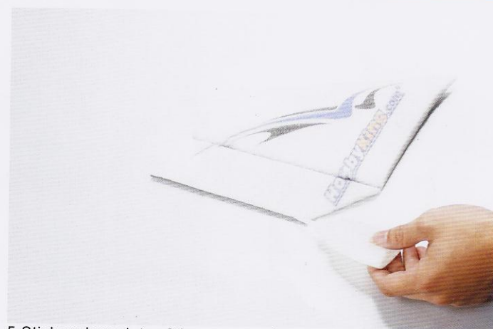
5. Stick carbon plate of the servo surface.
