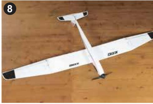
8 Apply the decals to the fuselage and wing as shown.
