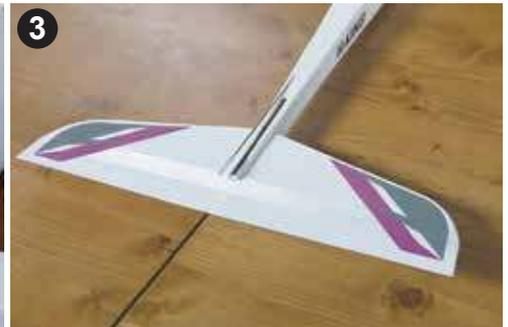
3 Trail fit the stabiliser on to the fuselage. Ensure it is parallel to the main wing.
