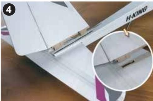
4 Trail fit the rudder on to the fuselage.
