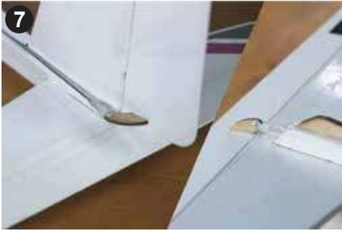
7 Attach the control horns to the control surfaces and apply CA glue as shown.
