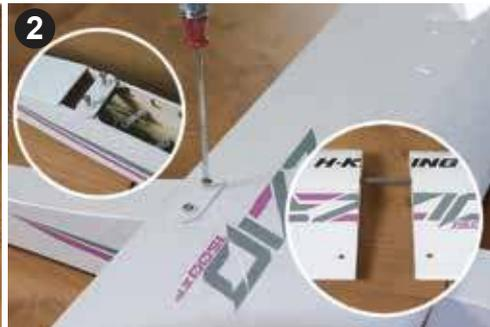
2 Put the wing together with the supplied wing spar and locate the wing on the saddle. Tighten it to the fuselage with the supplied screws as shown.
