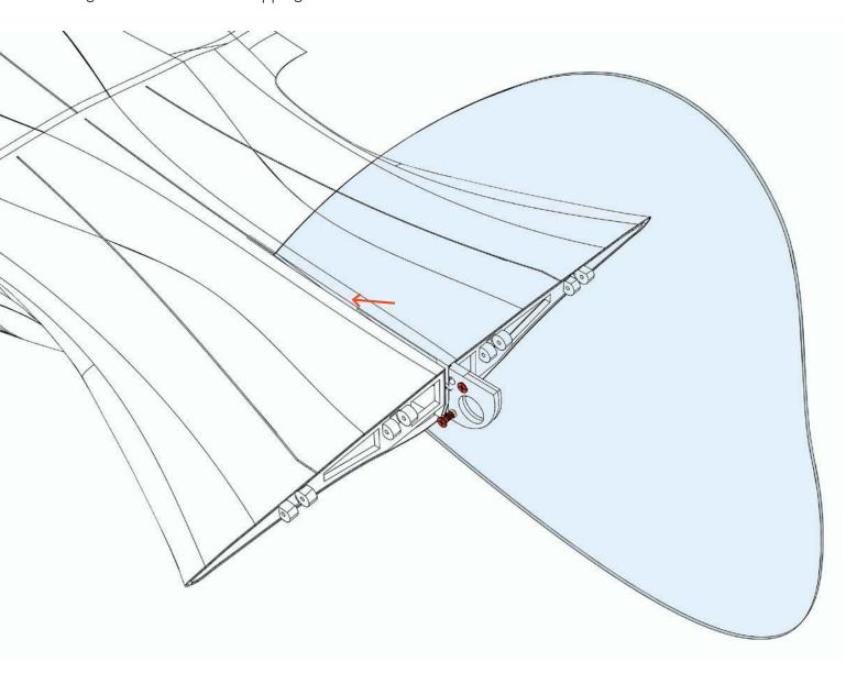
Fix the steel wire to the fuselage with a drop of CA glue.
