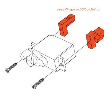
When the servo is installed, fix the cover (eagle-Servocovers-profile3.stl) with a tape.
