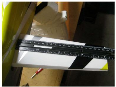
Insert the horizontal stabilizer into its slot. Do not glue yet. Center the stabilizer side-to-side in the slot using a ruler.
