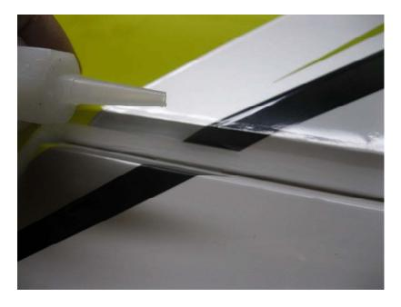
Glue the aileron hinges with two large drops of CA per hinge.
