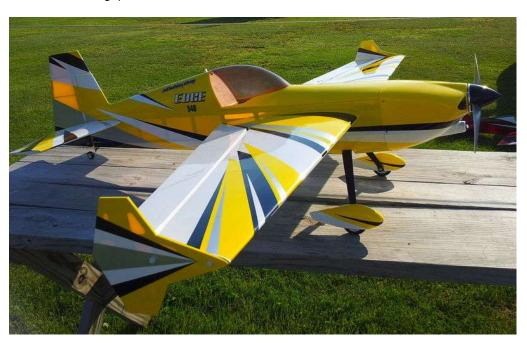
Balancing – Balance your Edge 540 3.75 inches or 95mm behind the leading edge of the wing where the wing meets the fuselage for your maiden flight. This is approximately on the forward edge of the carbon wing spar tube. Move the flight battery to balance as necessary. With lighter motors, the battery will have to be moved very far forward to balance. For 3D flight, move the CG slowly rearward as needed based on your preference.
