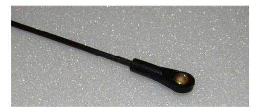
Assemble elevator pushrod as shown. Use thin CA on the ball-link to pushrod joint after installation to lock the ball-link onto the pushrod permanently. Slide carbon tube stiffener over pushrod.
