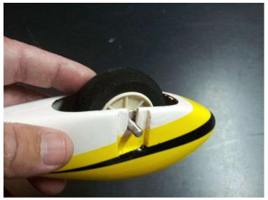
Slide one wheel/axle assembly into a wheel pant, and install the wheel assembly on the landing gear leg.
