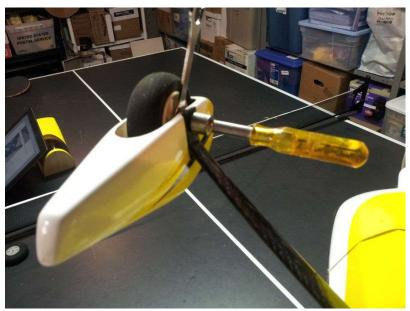
Tighten the locknut as shown to secure the assembly onto the gear leg. Repeat for other side. Install wood screw through drilled hole in gear leg into pant.
