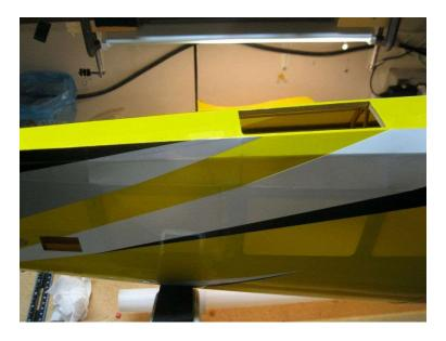
Remove a square or two of covering on the bottom of the fuselage behind the wing as shown, for cooling.
