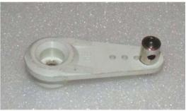
Install the pushrod connectors onto the servo arms as shown. Tighten the nuts just to a snug fit – the connector must be able to rotate after installation. Use medium CA glue on the nut to keep the connector from falling off due to vibration. Remember – the pushrod connector must be able to rotate so that the servo arm can move.
