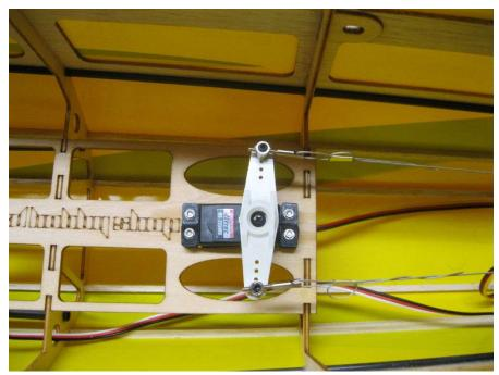
Mount the rudder servo and assemble the connectors onto the rudder servo arm as shown. Note that the connectors must be free to rotate on the servo arm. We use CA to lock the nut on the bottom of the connector for this reason.
