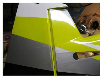
Install rudder onto fuselage and apply 2 large drops of thin CA to each hinge.
