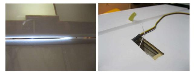
On the bottom of the wings, locate the servo cutout and aileron control horn slot. As with the elevator and rudder, shining a bright light such as an LED flashlight will help discover the slot. Remove the covering over both. Glue the horn into the slot with a generous amount of medium or thick CA. Use the string in the wing to pull the servo wire through the wing.
