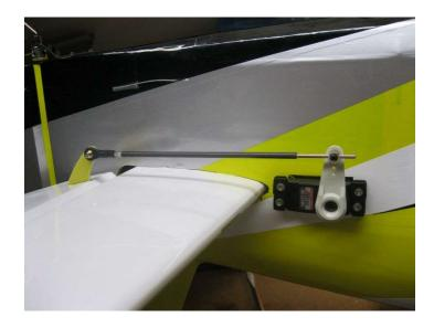
Install elevator servo with servo output spline toward front of plane and install arm and tighten pushrod connector.
