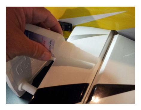
Install the elevator half with the fiberglass joiner rod onto the stabilizer. Makes sure it flexes easily at least 45 degrees up and 45 degrees down. Apply thin CA glue to the hinges, 2 large drops on each.
