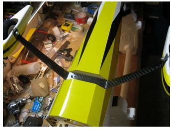
Attach the gear to the fuselage with short 3mm screws, use loctite.
