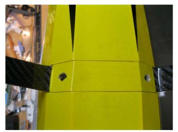
Install gear cover plate as shown, with clear tape, thick CA or epoxy glue.
