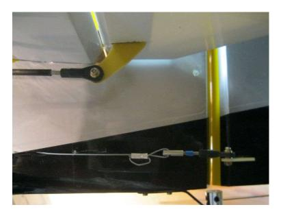
Assemble the pull-pull wires onto the rudder horn as shown, double-looping the wire through the brass crimp sleeve before crimping. Crimp the brass crimp sleeve tightly with pliers and apply a drop of thin CA to the crimp. Be SURE to use medium or thick CA to lock the 2mm nuts on the rudder control horn. Feed the wires into the fuselage slots and forward to the front of the fuselage. Cross the wires once so they make an X inside the fuselage.
