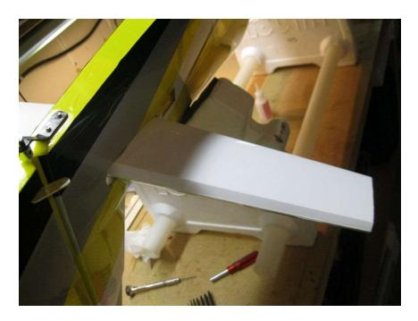
When stabilizer is centered and aligned, drip Thin CA glue onto the stab-to-fuselage joint top and bottom. NOTE: We do not remove any covering form the horizontal stabilizer. This keeps the stabilizer strong, and thin CA makes an excellent joint to covering material. If your stab joint is not tight enough for thin CA glue, or if you have to trim the opening to align the stab, you can use thick CA glue as well.
