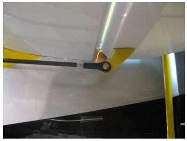
Install elevator pushrod onto horn as shown. Tighten the ball-link to the elevator horn using a 2mm screw, washer, and nut. Once the 2mm screw and nut are tight, use medium or thick CA glue to lock the nut in place so it cannot rotate. Make sure the 2mm screw and nut cannot come loose in flight.
