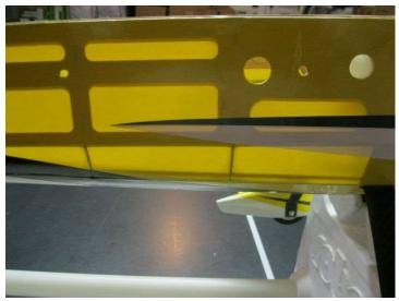
Remove covering over wing spar tube hole and wing pin holes in fuselage as shown.
