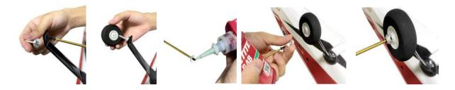
6. Install wheel cowls, tighten screws.
