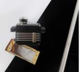
5. Remove black rubber ring from the wing side, pass aileron servo wire into the black rubber ring and secure it to the original position.
