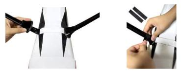
5. Install wheels, Secure wheels with gasket and screw. (Apply glue to screws)
