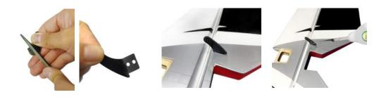
3. Remove the secured plate used for filling the horizontal tail slot, insert the horizontal tail into fuselage, please take note that it must be fully inserted into the fuselage.
