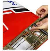
10. Unscrew the retaining screws on the wing, install wingtip.
