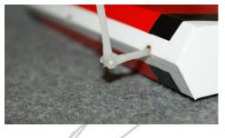
**NOTE:** Make sure to align the hinges by flexing them to the side 90 degrees and fully inserting.
