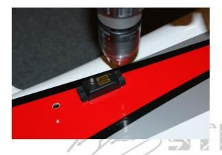
•Remove the servo and thread a servo screw in and out of each hole. Then apply 2 drops of thin CA to each and allow the CA to soak in and fully cure.
