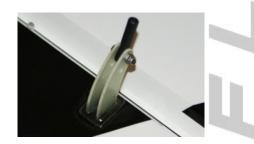
•Locate the servo pocket and remove the covering. Then drop the servo into place and drill for the servo screws with a 1/16" drill bit.
