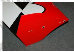
•The wing tips are easily secured with magnets and tabs which lock them in place.
