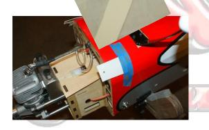
•Install the cowl, mark the mounting locations, and remove to drill. Drill a 1/8" hole in each location.
