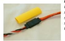
From the Pro: Use heat shrink tube to secure the servo lead to the extension.
