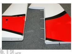
•Carefully align the hinge pins to the bores as you install to the fuselage and remove any
