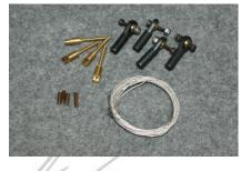
• Route the pull-pull cables from the slots in the rear of the fuselage to the rudder servo tray. At the rudder, slide a crimp onto the wire and loop the cable thru the link and back into the crimp with a loop as shown to hold the end in place for each side.
