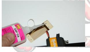
•Install the servo with the output to the leading edge, pulling the wire lead out to the root of the wing.
