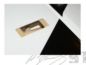
**From the Pro:** When removing the covering leave 1/8-1/4" of covering to be ironed down into the servo pocket. This makes for a much cleaner and more fuel-proof servo cut-out.
