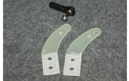
•Using the included linkage hardware, join the two horns as shown. Then mix a small batch of 15 min epoxy and coat the inside of the slots. Lightly coat the ends of the control horns and insert them into the slots, angled toward the hinge line.
