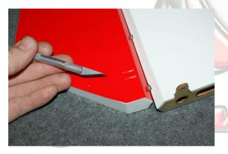
•Scuff the glue surface of the control horns using coarse grit sand paper or a rotary sanding tool.
