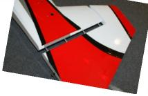
•Ensure the rudder moves freely bevel to bevel to allow maximum deflection and set aside to cure.
