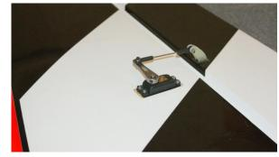
•Assemble the control rods to 3.25" length making sure the turnbuckle is centered with room to adjust both ends.
