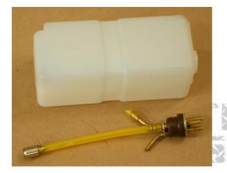
•The fuel tank utilizes a 3-line setup and is configured as shown above inside the tank.
