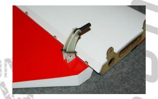
•You should have minimal squeeze out and a small fillet will form at the base of the horns. Clean up any excess with denatured alcohol.
