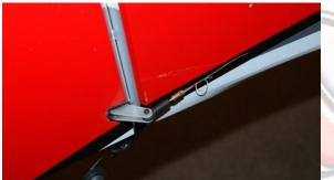
**NOTE:** Make sure the ball link is threaded in the center of the adjustment range (about ¾ of the thread) to allow even adjustment.
