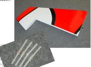
•Coat the pivot of each hinge with petroleum jelly all the way around working the hinge back and forth to ensure full
