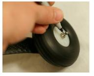
•Trim the axle, leaving the mark visible allowing 1-2mm excess to remain and file a flat as shown for the wheel collar.
