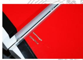
•Scuff the glue surface of the horns using coarse grit sand paper or a rotary sanding tool.
