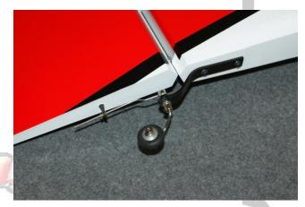
From the Pro: File a flat spot for the wheel collar on the wire and use medium thread locking compound to install the setscrews.
