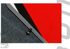
•There are blind nuts preinstalled for the tailwheel bracket. Locate the blind nuts, align the tailwheel assembly and install the screws using a thread locking compound.
