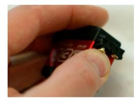
From the Pro: Use heat shrink tube to secure the servo lead to the extension.
