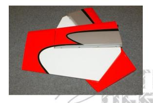
**From the Pro:** Some pilots prefer to seal the hinge gap. If you wish to do this, it is best to do it now before anything is installed to the elevator.
