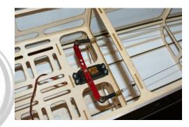
**NOTE:** The cables should cross inside the fuselage as shown when installed to the servo horn.
