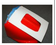
•After the initial cutouts are complete, test fit and adjust as needed until the cowl fits without any rubbing and a minimum 1/8" clearance.
