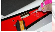
•Next, install the servo with the output to the rear, pulling the wire lead into the fuselage
