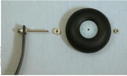
**NOTE:** The inner wheel collar will properly space the wheel for the wheel pant.
