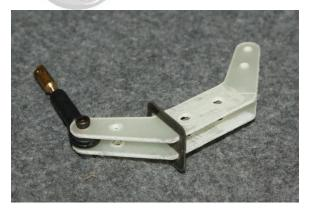
•Then mix a small batch of 15 min epoxy and coat the inside of the slots. Lightly coat the rudder control horns and insert them into the slots, angled toward the hinge line as shown.
