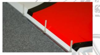
You should have some epoxy squeeze-out as the pin is inserted. Be careful to pull the excess epoxy away from the hinge point and not work it into the pivot.
