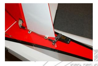
From the Pro: It is best practice to use a small washer on the outside of the ball link on the servo. This will prevent the ball joint from slipping off under load.
