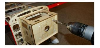
•Next, temporarily mount the motor in place to mark for the throttle linkage, fuel lines, and any ignition cable routing.
