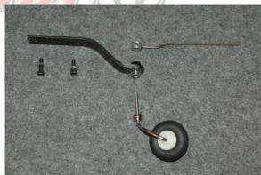
•Install the tailwheel bushing to the carbon fiber mount. Then install the wheel to the wire using the wheel collar and then secure the assembly using the upper retainer.
