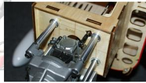
From the Pro: The throttle arm on the carb and the servo horn should be of the same length to allow full servo resolution and better/finer throttle control.
