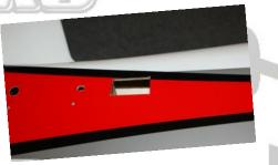
**From the Pro:** When removing the covering leave 1/8-1/4" of covering to be ironed down into the servo pocket. This makes for a much cleaner and more fuel-proof servo cut-out.
