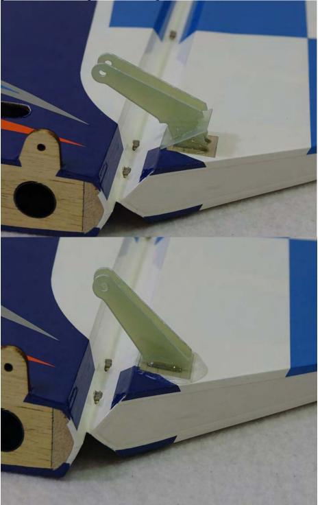
8. Wipe away the excess epoxy with a paper towel soaked in denatured alcohol, making sure to do a good job of cleaning the area. Insert a 3mm bolt and ball link into position and confirm proper alignment
