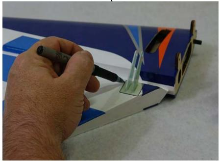
2. Remove the horn assembly and use your #11 blade to remove the covering from inside the ink line that you traced around the control horn base. Wipe away the ink line with a paper towel soaked in denatured alcohol.
