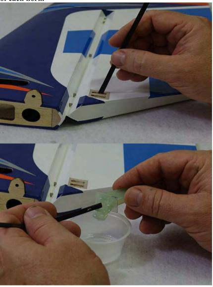
7. Insert the control horns into the slots and ensure that the horns are properly seated against the base plate and the base plate is flush against the control surface.
