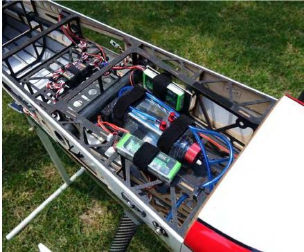
30. Mount your ignition to the interior side of the motor box lid and secure the lid with 4 screws. Next use a rotary tool to cut the cowl to clear the cylinder head, mufflers and make an air exit. Take a minute to add some thick CA or Epoxy to the intersection of the cowl and plywood cowl ring.
