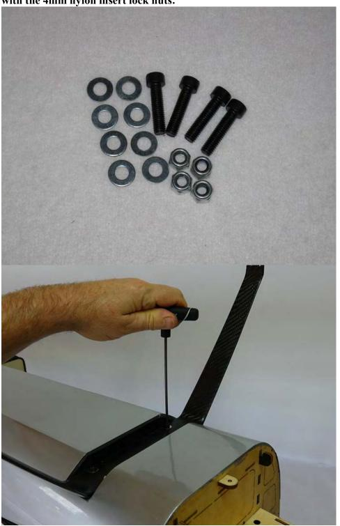
13. The landing gear fairings add a nice scale touch to the aircraft. Slide the fairing onto the gear and up against the fuselage. Secure the fairing to the gear with "Goop" silicon glue. Use blue painters tape to
