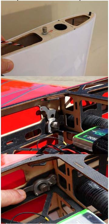
36. Included with your Edge are a set of Side Force Generators (SFGs) along with 2 clear spacers to be installed between the SFGs and wing tip to prevent them from interfering with aileron movement. They are to be installed using the supplied white thumb screws threaded through the holes in the SFG, through the clear spacer and into the pre-installed blind nuts in the wing tip.
