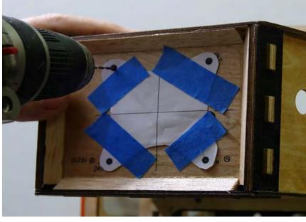
21. The distance from the front face of the motor box to the motor drive washer is 172mm or 6.8 inches (this is the length of the DLE-61, the longest of the engines recommended). Because the DA-50 is the recommended motor we have included a set of machined aluminum standoffs to be used in conjunction with the stock 2.5" standoffs included with the DA-50 to achieve the proper spacing.
