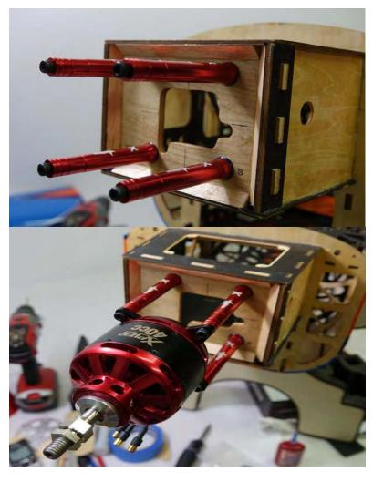
\*\*\*Please note that we removed the laser scribed panels in the F1 former in our electric powered airframe to allow cooling air to reach the batteries\*\*\*
