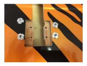
Enlarge the hole for the wheel a little bit (ca. 5mm to 8mm). This is due to the fact that the new style wheels are a little larger and better suited for grass runway operation.
