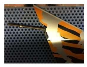
Mount the servo and the push rods as shown on the photo on the right. Attach the ball links to the aluminum control horn and clamp the control horn on the carbon axle.
