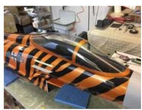
Paint the cockpit parts of and install the part with the pilot seat first, than the part behind.
