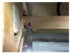
You may have to grind the hole in the rear balsa former to allow the thrust tube to fit through. This hole might be slightly smaller because it would fall apart in the production process before it is glued into the fuselage.
