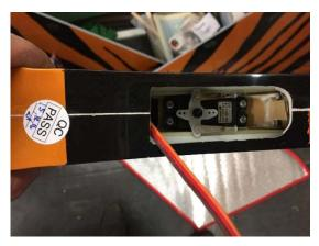
Then adjust the length of the threaded rods, solder the threaded ends on and install the linkages to the servo.
