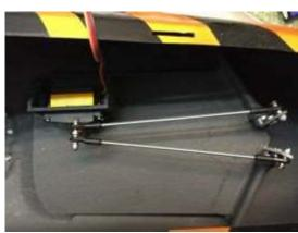
Use the panel line on the fuselage to adjust the neutral position of the canard.
