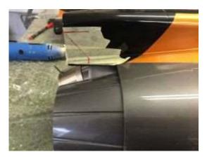
Cut 2 circular openings in the rear former to help to get the cooling air out of the fuselage.
