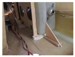
This picture shows the smoke tank. A 1 liter Coca Cola bottle fits perfectly into the fuselage-back.
