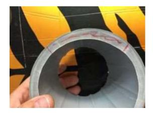
Cut out this part from the fuselage for 3D thrust tube support.
