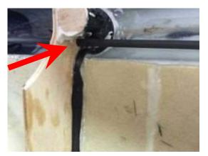
From some scrap balsa created a support for the vector push rods. It is enough if they are supported one at about half the length.
