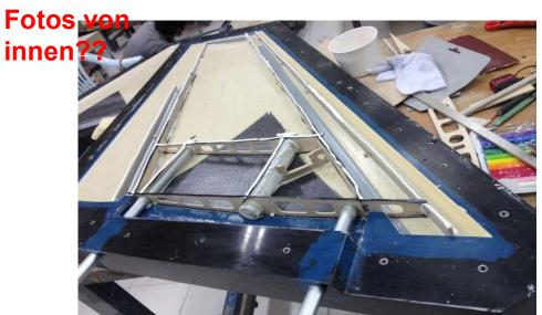
The fuselage and the wings are made of total area sandwich technology (TAVS) and are reinforced with carbon in the highly stressed areas. Carbon reinforced gear formers are installed and alligned.
