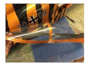
Glue the canopy into the frame (e.g. with silicone or 30 min epoxy) and position it with magnets.
