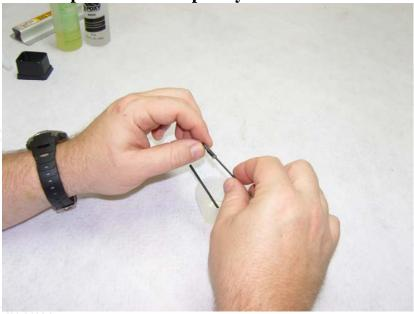
3. Use a paper towel to wipe away most of the excess epoxy, leaving a small fillet between the carbon pushrod and ball link. Position the pushrods vertically while they cure as illustrated so the fillet remains in position. DO NOT use CA for this bond!
