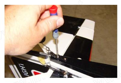
21. Secure the tiller using the provided screw, but do not over tighten as the tiller should be able to move on the screw as the ruder is deflected.
