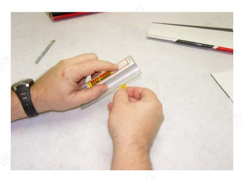
6. Use a glue tip on your bottle of medium CA and apply glue to the slot as well as to both sides of the control horn. Insert the control horn into the slot and make sure it seats properly against the surface of the aileron.
