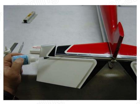
18. Remove the covering over the slot in the lower left side of the rudder where the rudder control horn will be installed. Scuff the portion of the control horn that will glue into the surface and secure the rudder control horn with medium CA.
