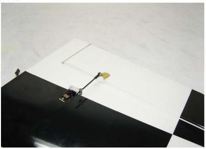
12. Secure the carbon pushrod to the EZ connector with the provided set screw. Take care not to over tighten the set screw and crush the carbon rod. Once you feel the set screw engage the carbon pushrod another 3/4 to 1 turn will supply adequate pressure to retain the pushrod. Make sure that the servo arm is perpendicular to the servo case when the aileron is in the neutral position.
