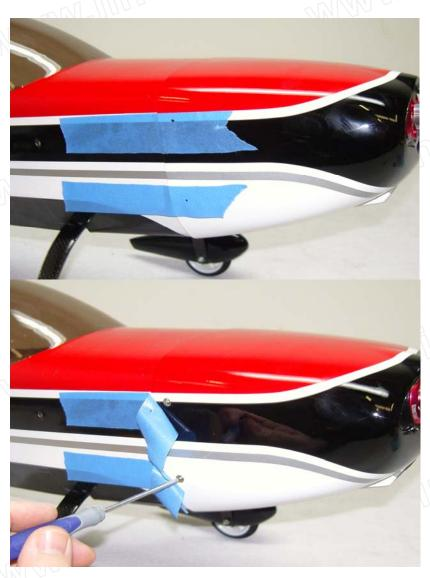
27. There is a laser cut opening in the bottom of the fuselage under the rear of the canopy. Use a sharp hobby knife to remove the covering from this location to allow cooling air to exit the fuselage.
