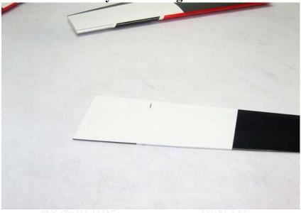
5. Scuff the portion of the control horn that will be glued into the aileron with sandpaper.
