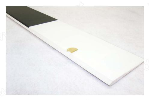
7. Remove the covering from the aileron servo location and make sure the hinges are centered in their slots.
