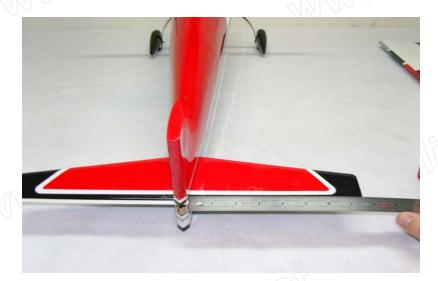
16. Remove the covering over the left slot on the bottom of the elevator where the elevator control horn will be installed. The elevator horn is the one with the shortest shank that is glued into the surface. Scuff the portion of the control horn that will insert into the elevator with sandpaper. Secure the control horn with medium CA.
