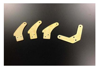
Note: if installing the rudder servo in the aft position (for push-pull), you may cut off one side of the rudder control horn. Otherwise, install the double control horn for pull-pull installation.
