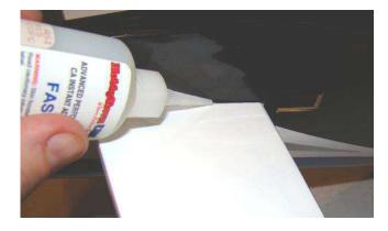
Apply medium CA into the slot in fuselage and install vertical stabilizer.
