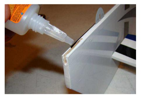
Install second elevator onto elevator joiner rod and slide hinges into stabilizer. DO NOT GLUE HINGES YET. Allow joiner rod to cure.
