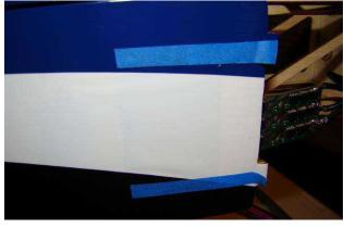
Install cowl and align, use tape to hold the cowl in position while you work. Use the tape strips to locate the position for the holes in the cowl. Use a small drill or a hobby knife to make holes in the cowl.
