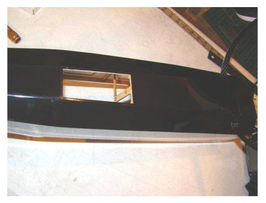
Remove covering over wing spar hole, wing bolt hole, aileron wire hole, and anti-rotation pin hole as shown in side of fuselage on both sides.
