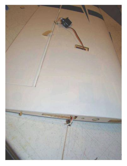
Install the servo using the servo screws which come in the servo package. Install pushrods and servo arms as shown.
