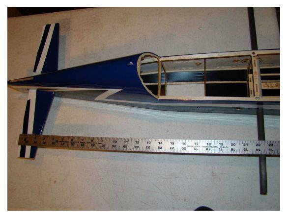
Drip thin CA glue into the stabilizer-fuselage joint. Do not remove any covering from the horizontal stabilizer.
