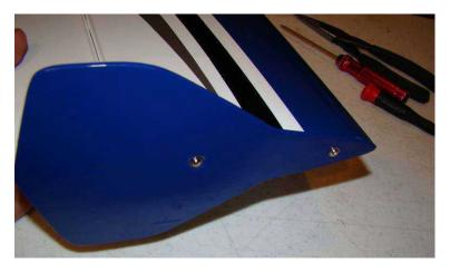
Attach wings to fuselage with nylon wing screws. NOTE – the carbon wing tube is designed to be removable, and is not meant to be glued in place.
