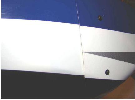
Align covering stripes on ailerons with stripes on wings. Apply two large drops of thin CA glue to each aileron hinge. Allow to cure.
