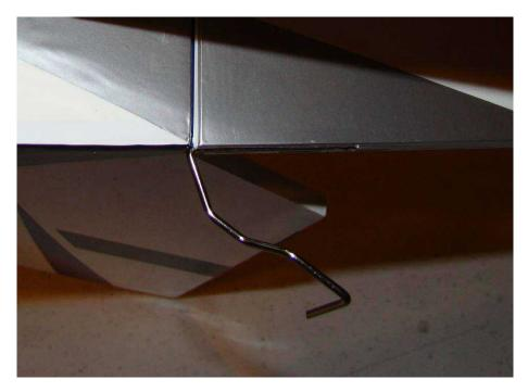
Install tailwheel bracket with two small wood screws. Check for free swinging of rudder. Adjust bracket as necessary to allow rudder to swing freely. Install tailwheel and tighten tailwheel collar with 1.5mm allen wrench.
