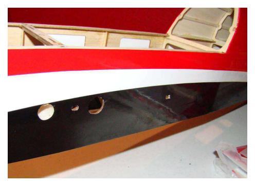
Remove the covering over the horizontal stabilizer opening and servo opening on both sides of the fuselage as shown.
