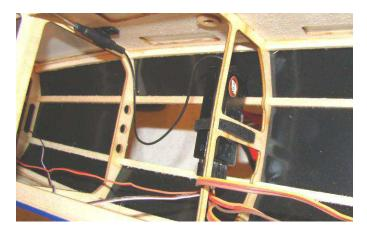
The cowl mounts using 4 small wood screws which screw through the cowl into small plywood rectangles at the front of the fuselage. In order to know where to make the holes in the cowl for the screws, place tape strips on the fuselage over the plywood as shown.
