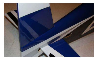
Drop a few drops of thin CA onto the elevator joiner rod at the factory joint of elevator and rod. Allow to soak in for a few minutes, then wipe off excess.
