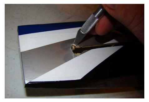
Insert horizontal stabilizer (note the color scheme on top). Use a ruler to square the stabilizer side to side as shown.
