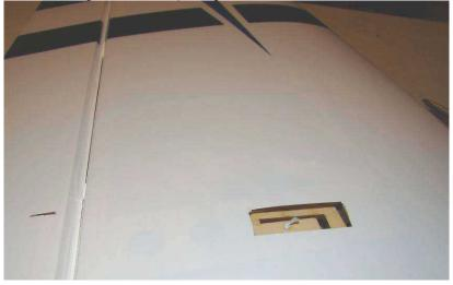
Install aileron control horn as you installed the other horns. Use the installed pull-string to pull the servo wire through the wing.
