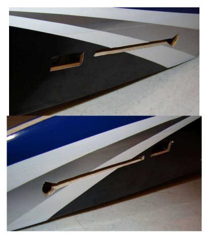
Trim rear section of stabilizer opening to ensure good clearance for elevator joiner.
