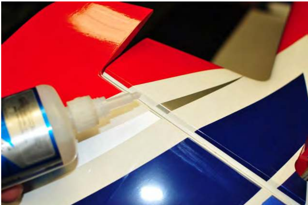
Install rudder using two generous drops of thin CA on each hinge
