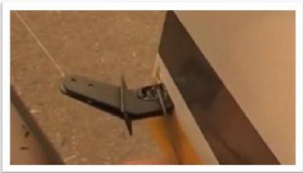
Mark the center of the rudder along the hinge line.
