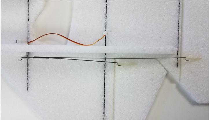
**Adhere servo wires-** Push RH servo wire through lower fuselage to LH side. Flatten and route the servo wires in the slots under the main carbon spar, tape into place. I like to use ½" wide 3M blenderm tape, it sticks well to the epp, and is nearly invisible once applied.
