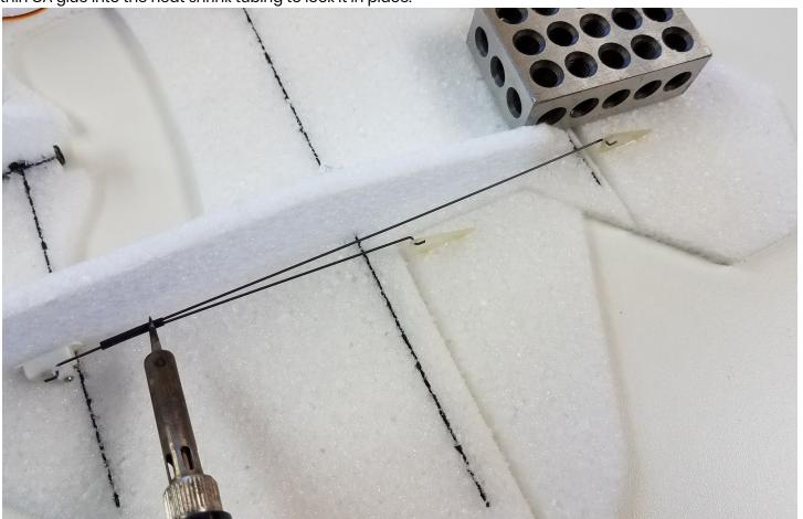
**Connect pushrods to servos-** Once completed, your installation should look like this, with the other side being a mirror image. Note that all of the pushrod wires are to the inside of the control horns and the servo horn. This eliminates the elevon pushrods from contacting the ailerons when deflected.
