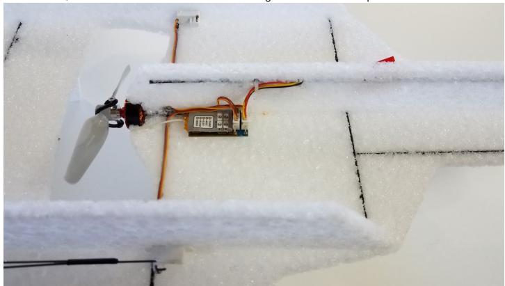
**Center of Gravity-** should be located \( \)" ahead of the front spar.
