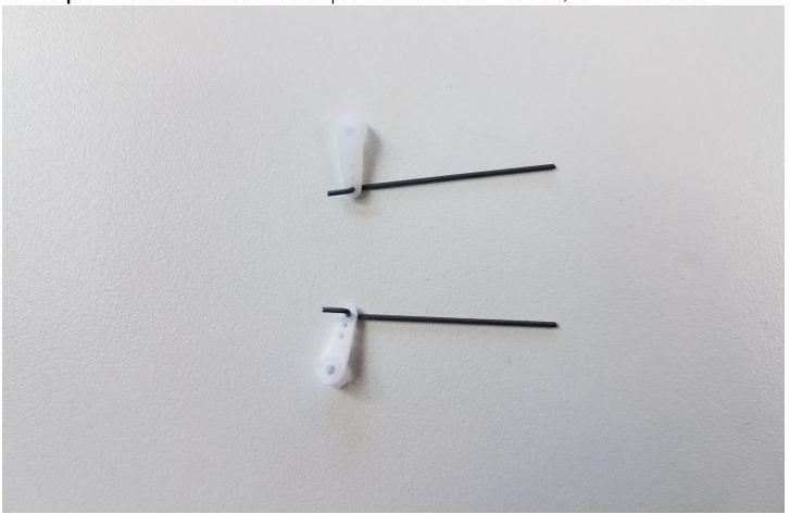
**Connect pushrods to servos-** Push each servo arm onto it's servo so it is exactly vertical, slide ¾" length of heat shrink tubing over all three pushrod pieces.
