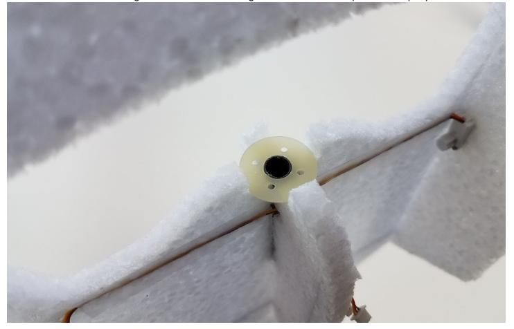
**Install motor and esc-** Install the motor with the wires exiting as shown on the aircraft's RH side. If using a tube mounted motor, apply a very small amount of medium CA glue and insert motor tube into carbon motor mount. If using radial mounted motor, use screw supplied with the motor and install motor to radiall mount. Use supplied zip tie and predrilled holes in lower fuselage to secure ESC. Push receiver wire though hole in lower fuselage to the aircraft's LH side.
