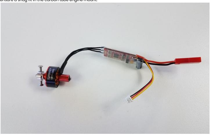
**Install motor mount-** If using radial mounted motor, glue radial mount into place with epoxy.
