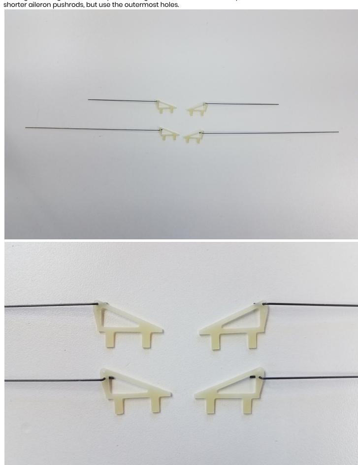
**Install pushrods-** Glue the assembled pushrods and control horns into the precut slots on the elevons and ailerons. Keep the pushrods to the inside of the control horns.
