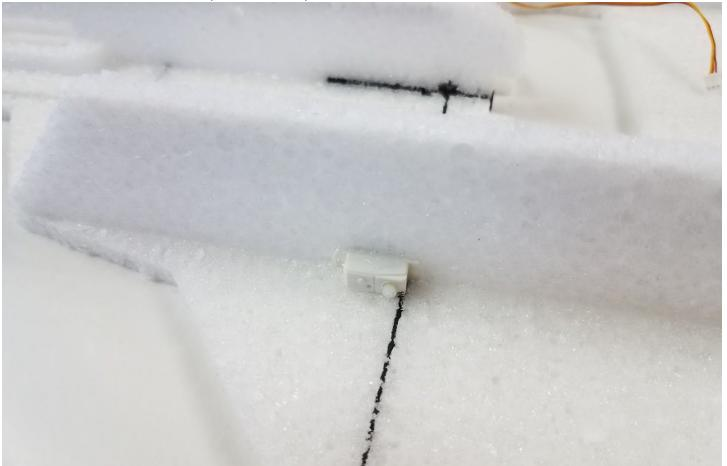
**Assemble pushrods-** insert the longer elevon pushrods into the innermost hole on two control horns, making both a right and a left by alternating which side of the horn the pushrod is on. Do the same for the shorter aileron pushrods, but use the outermost holes.
