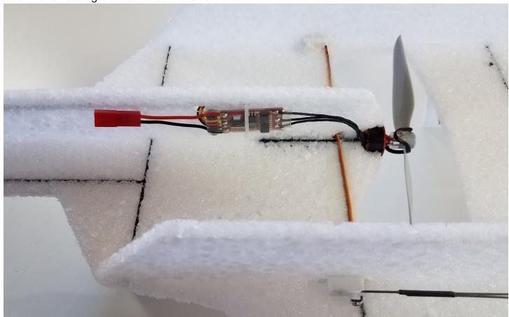
**Install receiver-** Carefully plug in both servos and the esc to the receiver. Bind receiver to your transmitter. Check function of servos and esc to ensure that you have everything plugged in properly. Carefully route receiver wires, and stick receiver to the bottom of the wing with double sided tape.
