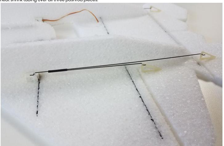
**Connect pushrods to servos-** While ensuring the fuselage, elevons, and ailerons are all aligned flat with your work surface, use a soldering iron or other means to shrink the heat shrink tubing. Wick a small amount of thin CA glue into the heat shrink tubing to lock it in place.
