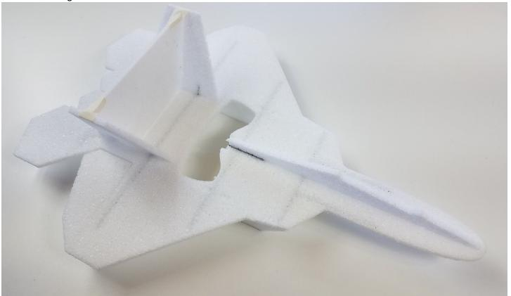
**Paint-** Now is the time to paint if desired. There are many different ways to paint an EPP aircraft. Basic acrylic craft paint work great. One of the keys to a good paint job on this type of aircraft is to apply a minimum amount of paint and consequently weight. Airbrushes work best, but brushed work too. Some aerosol paints made for plastic also work very well.
