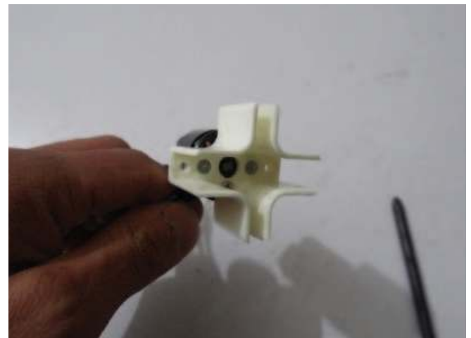
Assemble motor on motor mount using motor's screws.
