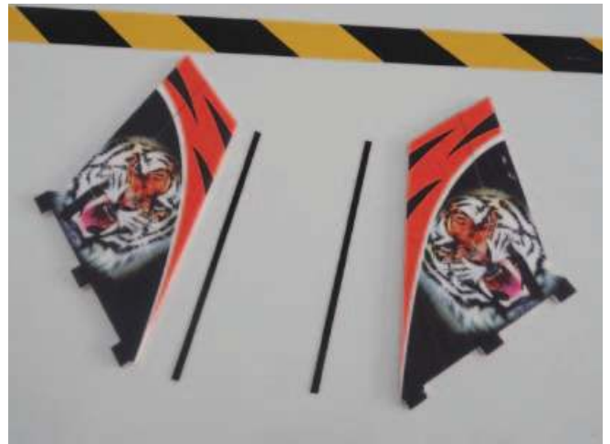
Stick the 2 pcs carbon strips on vertical tail using foam glue.
