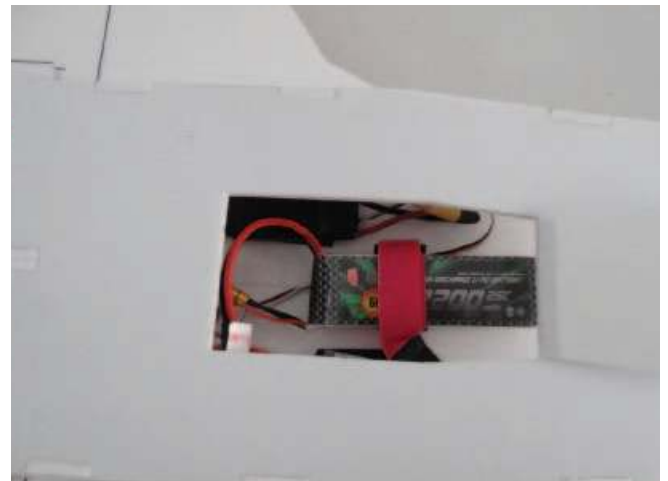
Use another hook and loop tape through the hole to fix battery.
