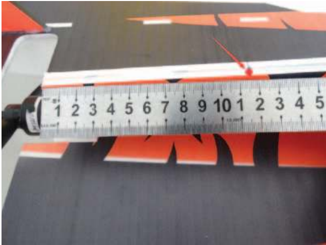
C of G is on the front of the motor mount 11.5cm as shown in the picture above.
