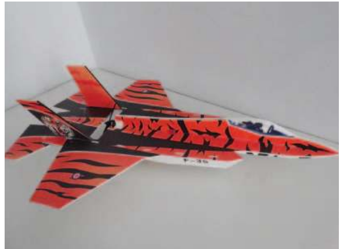
PP F35 just has tail control, so we need set delta wing mixed control on radio (Elevator and aileron mixed control). We advise set elevator parameter to 60/70 and set aileron parameter to 90/100 on radio.
