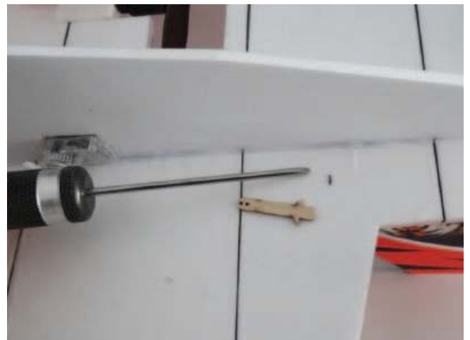
Install wood strip in the hole using No.502 glue.
