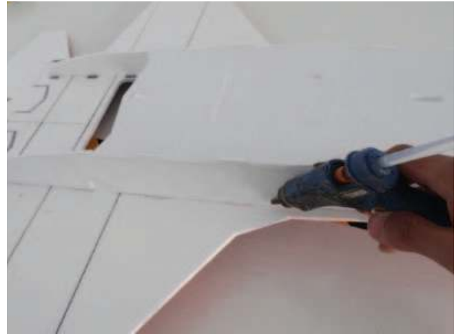
Also don't forget to reinforce vertical fuselage using hot glue sticks.
