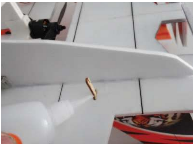
Install arm on servo and electrify all servos to make sure the arm perpendicular to servo. Then install arm screws. Install servo in the hole using hot melt glue.
