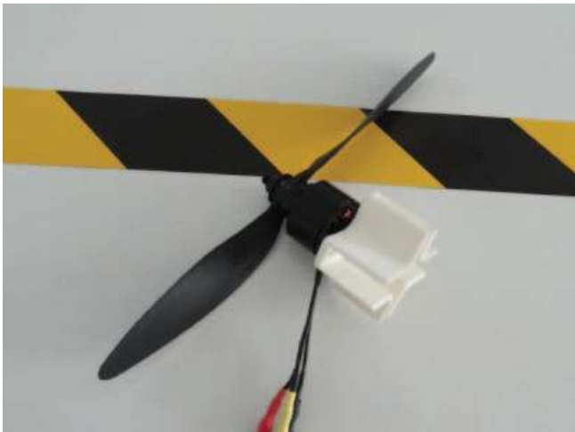
Assemble prop on motor. Notice the prop's direction.
