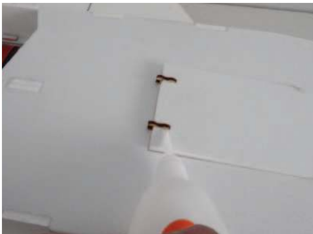
Install the 2 pcs wood clips in the bottom cover using foam glue.
