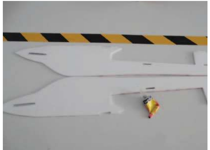
Applying foam glue on 2 pcs nose.
