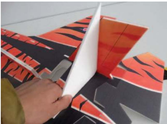
Install vertical tail on fuselage using hot glue sticks. Must use triangle foam board to make sure vertical tail's incline.
