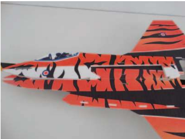
Assemble the nose on fuselage using hot glue sticks or foam glue, make sure the motor mount location must be flat!
