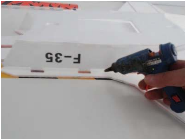
Then assemble vertical fuselage and bottom fuselage on horizontal fuselage using hot glue sticks.
