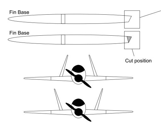
Note: The base of each fin incorporates a slight angle at the trailing edge which mirrors the swept leading edge of the control surface. If you choose the inward-facing fin arrangement you'll need to dry fit each, mark the cut position on the base, then trim to fit (as shown) before gluing firmly in place.
