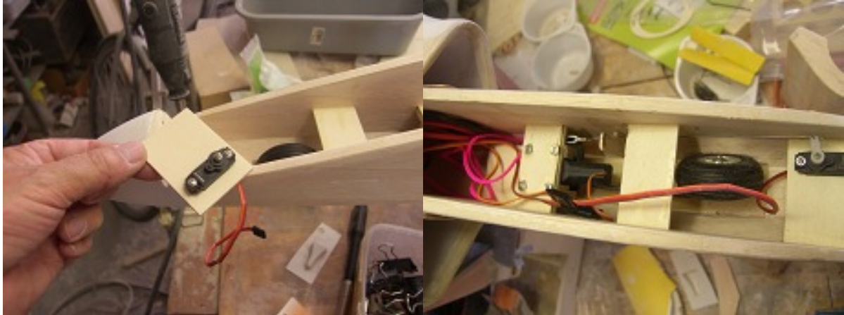
Place steering servo in RS4 place RS1,RS2 and RS3 , depending on your retract type you can have a top or bottom mount , , formers for bottom mount are also in the cut parts (RS6,7,8)
