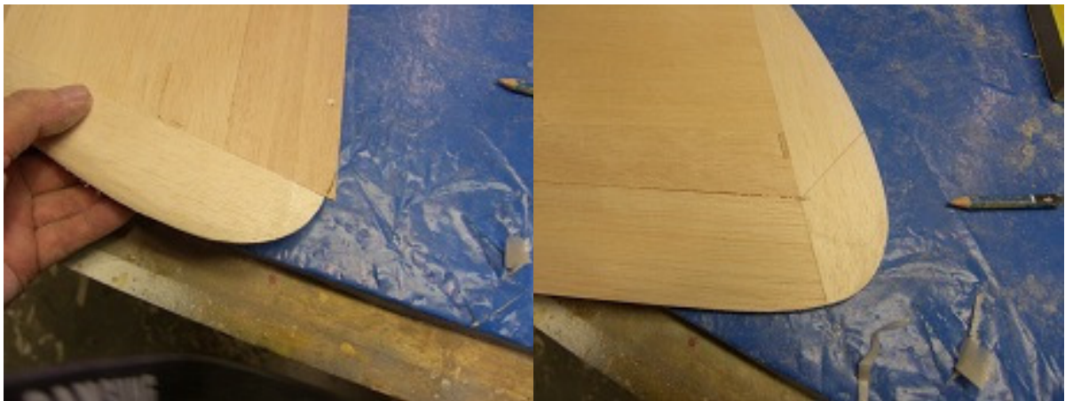
For the aileron tips you might want to use the scale outline, but this might not be handy when landing without a landing gear, we suggest for that that you use the straight aileron option.
