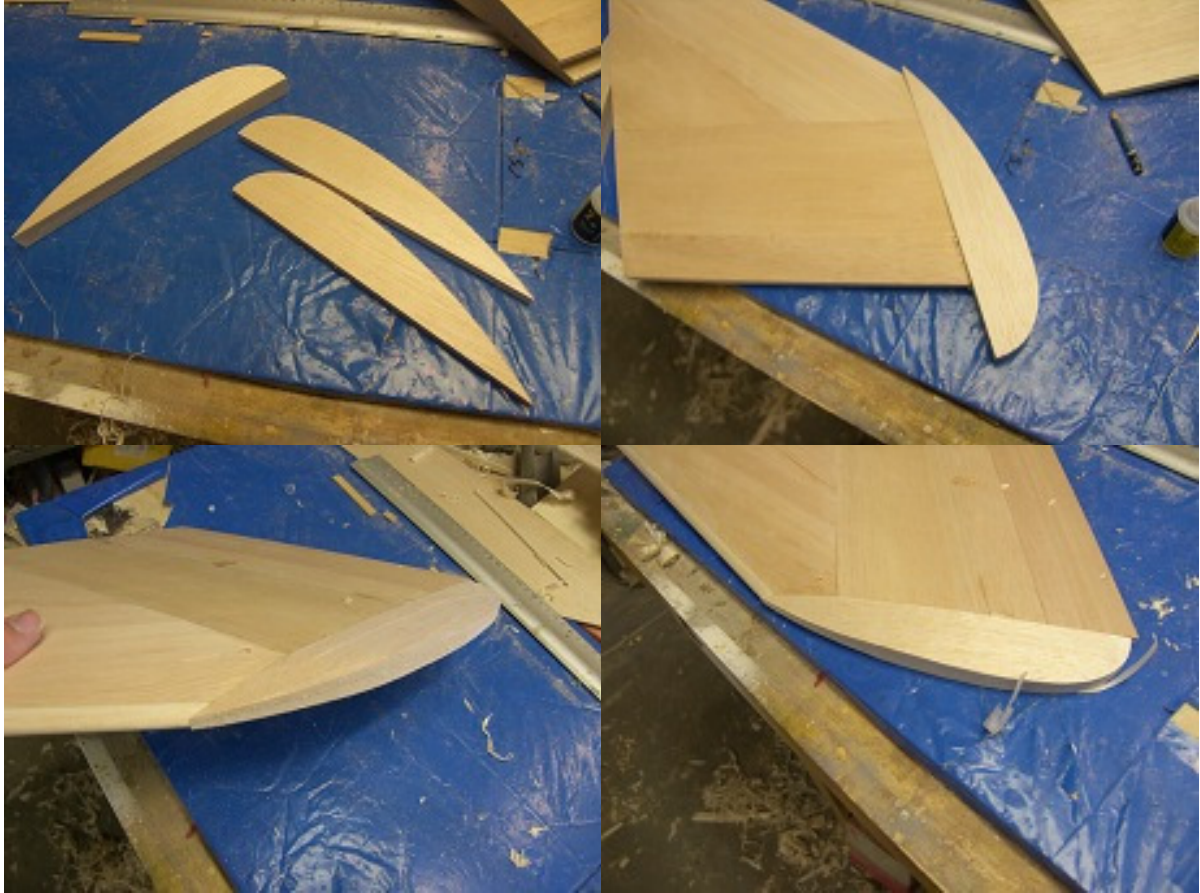
Sand trailing edge to fit tip
