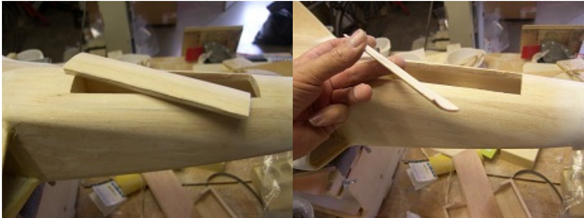
Place steering servo in RS4 place RS1,RS2 and RS3 , depending on your retract type you can have a top or bottom mount , , formers for bottom mount are also in the cut parts (RS6,7,8)
