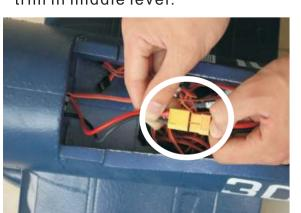
3. Connect power battery, adjust the elevator and rudder.
