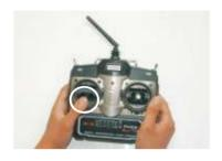
(9) Close the throttle on the transmitter before connecting battery otherwise the motor may operate.
