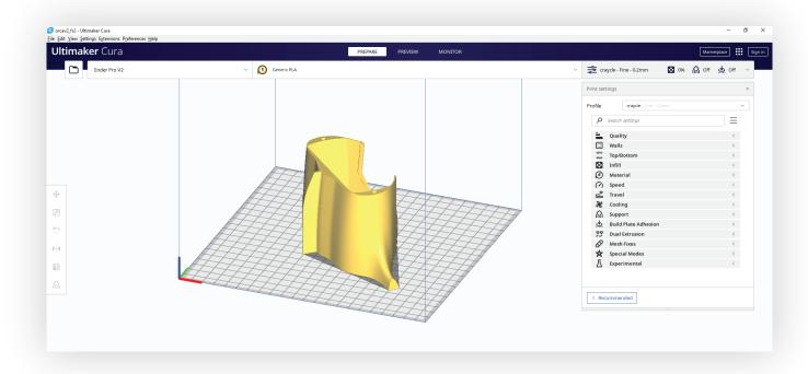
We pre-routed the model parts for you but still make sure the model parts are oriented at 45 degrees to the bed. This way X and Y axis works coordinated and you can get maximum surface quality. You can also set the Z seams to corners.
