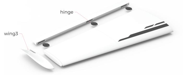
Now you can break the aileron from its tiny connections and re-assemble them using CA Hinges. Then you can glue the "wing3" part to its place. Avoid using excessive glue and spray on the hinges. The same process goes for the other wing.
