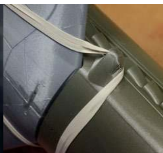
F2 & F4 for rubber banded wings
