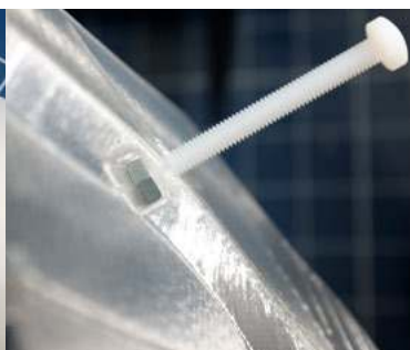
M5 screw and nut for wing
