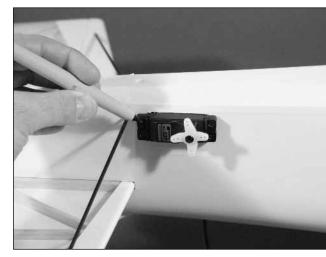
🗆 🗆 Step 4 Remove the servo and drill the holes for the servo mounting screws using a 1/16" drill bit.
