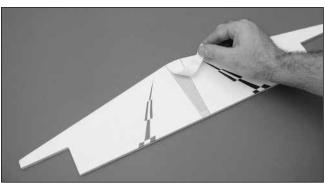
**Note**: Use care not to cut into the underlying wood and weaken the structure. Doing so will almost guarantee stab failure in flight, which is not a good thing.
