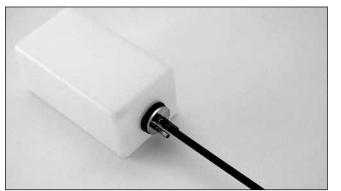
**Important**: Be sure to differentiate between the vent and fuel pickup tube. Once the tank is mounted inside the fuselage, it will be difficult to tell the tubes apart.
