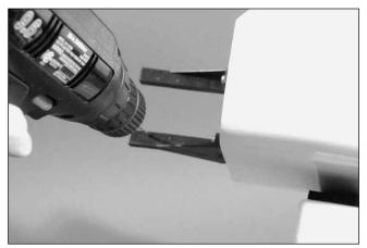
**Cool Tip**: Use a drill press for the best results. This makes holes perfectly perpendicular (square) to the mount.
