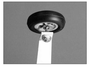
**Cool Tip**: Position the set screws on the wheel collars facing directly down. This way you can get to them later to position the wheel on the axle.
