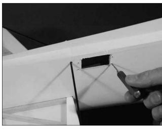
**Cool Tip**: Place a drop of thin CA onto each screw hole to harden the wood around the
