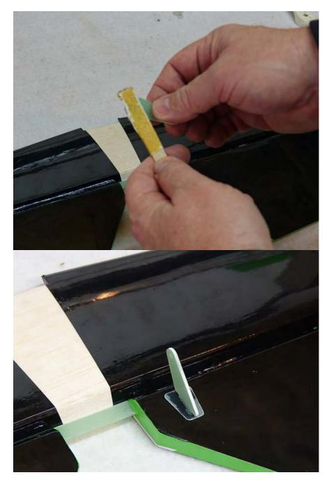
10. Slide the elevator onto the hinges and secure to the horizontal stab with several drops of CA at each hinge location. Be sure to use a fresh bottle of thin CA to ensure maximum penetration and adhesion.
