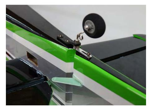
16. Place the tailwheel wire in the proper position, aligned with the rudder and lock into place with the set screws.
