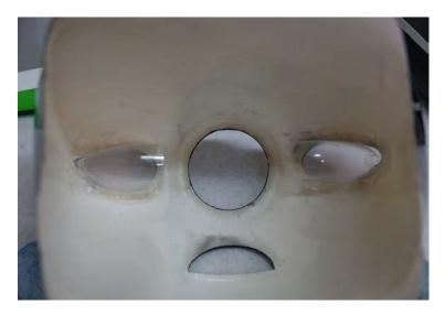
20. The holes for mounting the cowl are already pre-drilled at the factory. Place the canopy onto the fuselage and slide the cowl into position and secure with 4 3mm bolts and washers. In this picture we used the optional EF Xessories anodized black washers for an added touch of Bling. Be sure to use blue Loctite on each bolt!
