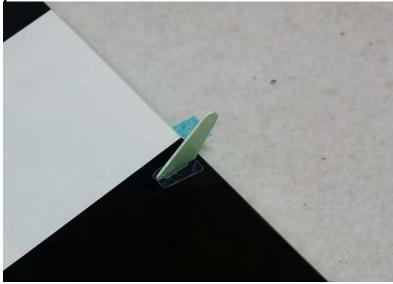
3. Center the hinges in their slots and slide the aileron into position making sure the outer tip of the aileron is flush with the wing tip and that there is no more than 1mm gap between the aileron and wing trailing edge. Apply a drop of CA at each hinge location on both the top and bottom side of the wing. Use a fresh bottle of thin CA and a fine glue tip for best results.
