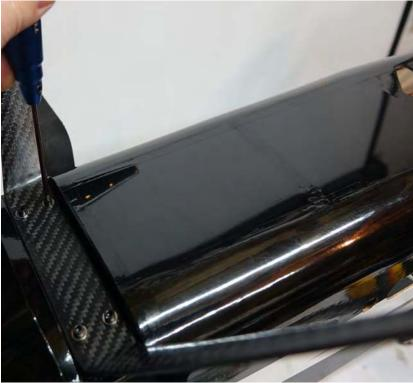
9. Next lets mount the horizontal stab. In preparation to do this we need to remove the Ultracote covered filler block at the rear of the stab slot. I also find it easier to go ahead and hinge the elevator and install the control horn before gluing the stab into place. Locate one of the control horns with the shorter shanks. Scuff the area that will be glued into the surface, slide it into the baseplate and glue into the precut slot with medium CA.
