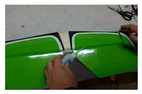
11. Slide the horizontal stab into position making sure to push it as far forward into the slot as possible. The alignment recess in the forward part of the stab will aid in proper positioning. Compare the stab with the vertical fin and make sure it is perfectly perpendicular. Adjust slot as necessary to achieve this and when satisfied with alignment secure the stab to the fuselage with a combination of thin and Medium CA.
