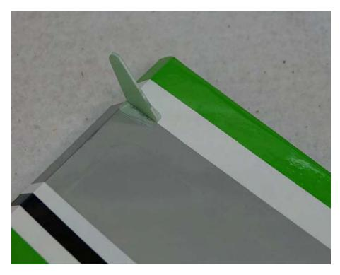
14. Using the same process as with the ailerons and elevator, slide the rudder onto the hinges and secure to the vertical stabilizer with thin CA.
