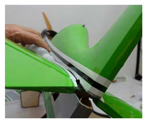
12. Once the glue securing the stab is dry glue the filler block back into place behind the stab.
