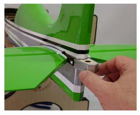
13. Scuff the shank on the rudder control horn and glue into position with medium CA as shown.
