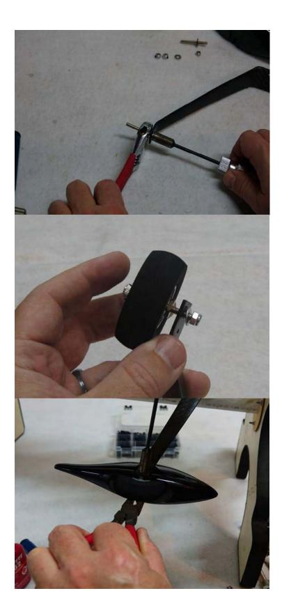
8. Secure the landing gear to the fuselage by inserting a 3mm bolt into a washer, through the carbon fiber gear and into the pre-installed blind nuts in the fuselage. Make sure to use a drop of blue Loctite on each bolt to prevent them from backing out. <u>Please note the carbon gear should sweep back in relation to the fuselage.</u>
