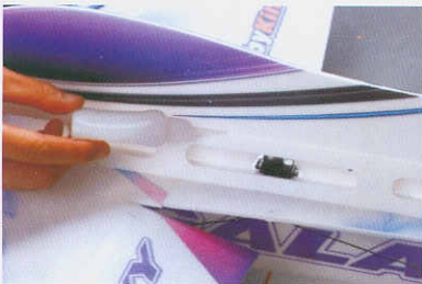
28. Fix the fuselage stringers to the fuselage. Note: Keep the fuselage and wing vertical, no distortion.
