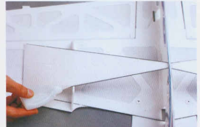
18. Apply some C/A to all the joints of carbon fiber rods and the wing strengthen foam.
