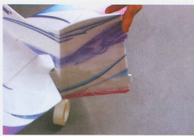
23. Fix the rudder to the fuselage with 3M magic tape.
