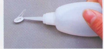
34. Glue together the contron horns and their backplates. (for aileron)
