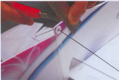
40. Cut a 40mm long carbon fiber strip and a 20mm slot on the bottom vertical fuselage as shown. Insert the strip into the slot, then apply some C/A to fix it. The strip is used as a tail skid.
