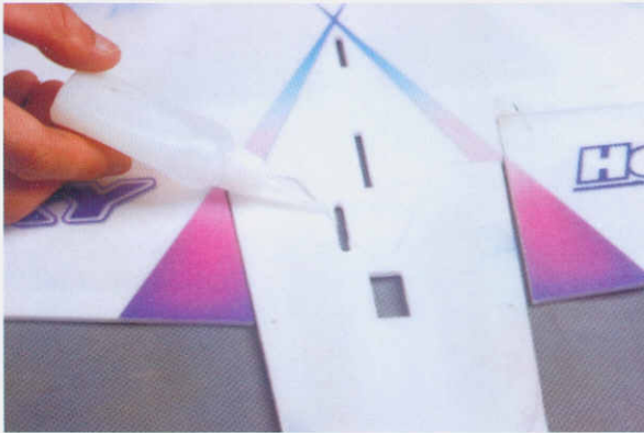
5. Key the rear of horizontal fuselage into the wing and apply some foam friendly C/A.
