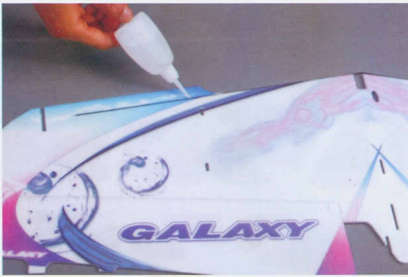
3. Glue 2pcs carbon fiber strips on the front of wing with some foam-friendly C/A.
