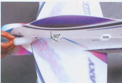
22. Key the upper vertical fuselage on the wing with some foam friendly C/A. Be vertical and no distortion.
