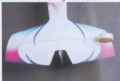
19. Fix the elevator to the fuselage with 3M magic tape.
