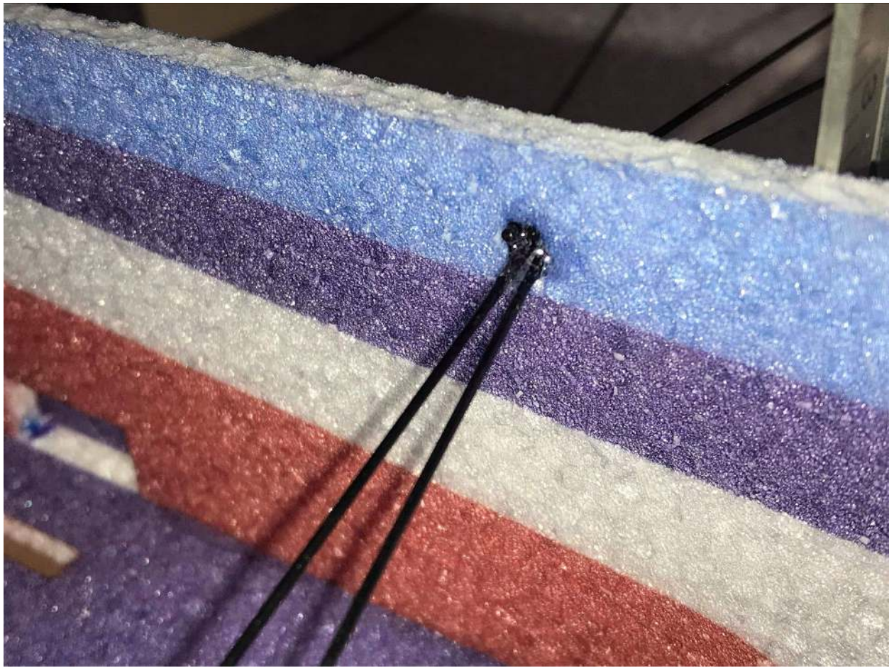
Shown above is the wing bracing glued into the bottom part of the fuselage.
