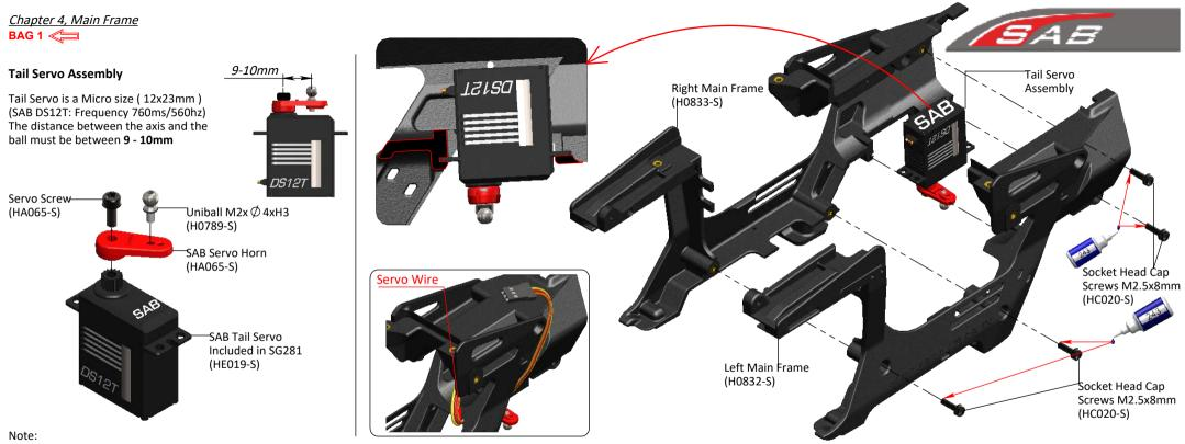
The tail servo is held in place by the tension created when the main frame is assembled; this means that there is no requirement to attach the servo directly with screws. The tail servo can be removed by loosening the screw that tensions the frame to the tail boom. There is no requirement to disassemble the frame completely. Page 5
