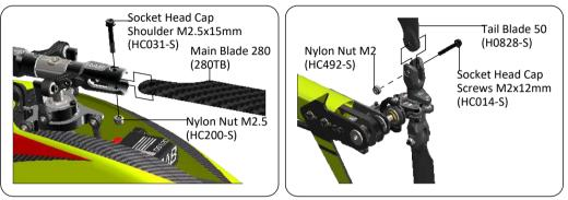
\*Check the collective and cyclic pitch. For 3D flight, set about +/- 13°.
