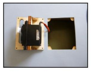
8) Set the aileron hatch in place and use a Phillips screw driver to install it with four wood screws.
