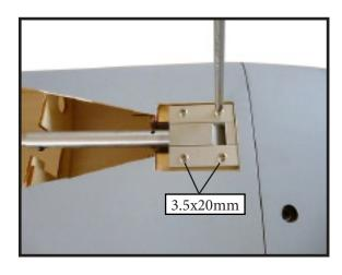
Install servo for wings gear.
