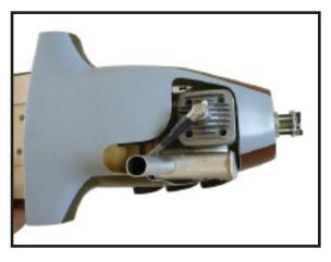
3) Assemble the wings temporary to mark for cutting cowling as shown.
