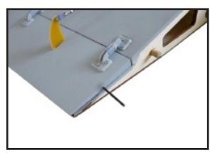
Slide the wing tube into the wing tube socket.
