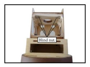
5) Attach the motor to the front of the electric motor box using four 4mm blind nut, four M4x20mm hex head bolts to secure the motor. Please see picture shown.
