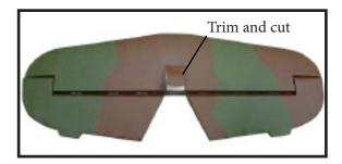
When cutting through the covering to remove it, cut with only enough pressure to only cut through the covering itself. Cutting into the balsa structure may weaken it.
