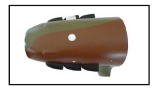
1) Tape the cowl to the fuselage using low-tack tape.
