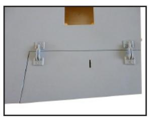
INSTALL FLAP CONTROL HORN FOR CENTER WING.
