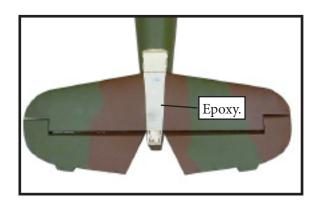
4) Slide the vertical stabilizer back inplace. Using a triangle, check to ensure that the vertical stabilizer is aligned 90° to the horizontal stabilizer.
