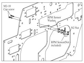
TSA RPM Sensor assembly means 2: ( only for left main frame assembly)
