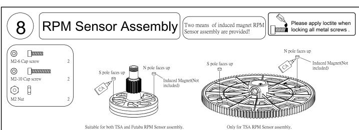
Suitable for both TSA and Futaba RPM Sensor assembly.
