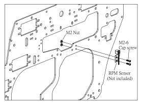
Futaba RPM Sensor assembly means : ( for both right and left main frame assembly)
