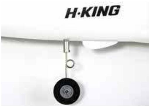
**Step 1:** Assembly of the nosewheel. Fit the nosewheel into the nosewheel steering collet with the spring at the back. Ensure the flat on the wire lines up with the M3 x 3mm grub screw in the steering collet. Use a hex wrench to tighten the grub screw.
