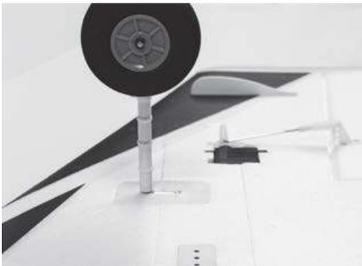
**Step 3:** Main landing gear. Install the main landing gear into the grooves on the main wings using the 2 x 8mm self tapping screws provided.
