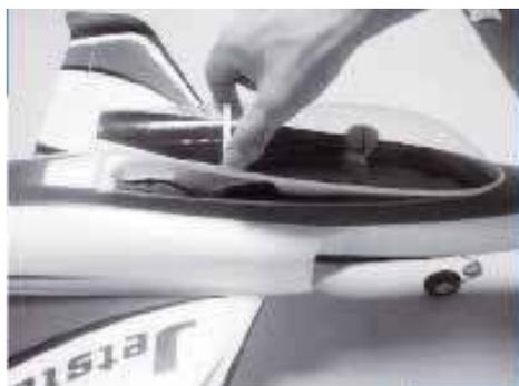
**Caution:** When opening the canopy carefully grip it close to the rear and gently ease it upwards. It is held down at the rear by a strong magnet and the front has a locating tongue.
