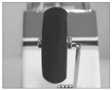
O 11. Locate two 4mm wheel collars and two 3 x 5mm set screws. Install the screws into the wheel collars. Slide a wheel collar and set screw onto the nose gear wire, followed by the foam nose wheel and another wheel collar and set screw. Tighten the set screw in the outer wheel collar onto the flat spot you filed on the end of the wire. Center the nose wheel and then tighten the set screw on the remaining wheel collar.
