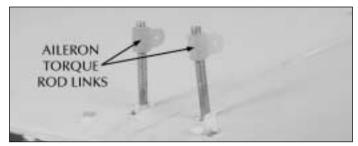
O 2. Locate two nylon **aileron torque rod links**. Thread them onto the aileron torque rods approximately 20 full turns.
