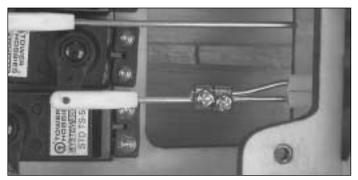
O 13. Locate two 4mm wheel collars and two 3 x 5mm set screws. Slide them over both of the elevator pushrods. Center both halves of the elevator. Then, tighten the set screws. Install the wire pushrod into the servo arm, retain the pushrod with a nylon pushrod connector and then install the servo arm onto the servo.
