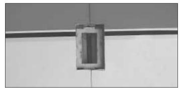
O 7. Glue the servo tray into the wing with 6-minute epoxy.
