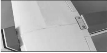
O 11. Temporarily bolt the wing to the fuselage with two 4 x 40mm bolts and two 4mm washers.
