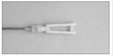
O 9. Locate the .074 x 16" [406mm] pushrod, threaded on one end. Thread a nylon clevis onto the threaded portion of the rod approximately 20 full turns. Install a silicone clevis keeper onto the bottom of the clevis.
