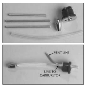
**O** 2. Assemble the components. Included in the fuel tank parts are three aluminum tubes. If you will be fueling your plane with a third line rather than filling the tank through the carburetor line, you will need to use the third aluminum tube. If not, assemble the tank as shown with a vent line and carburetor line. Once assembled, use a fine tip marker and mark the front of the fuel tank so you can identify which is the vent line and which is the carburetor line.
