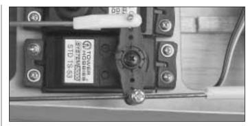
O 10. Insert the throttle pushrod into the screw-lock connector. Center the servo and then tighten the set screw against the pushrod wire.
