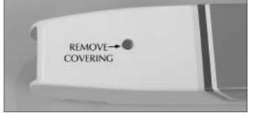
**O** 1. Locate the **fuselage**. Cut the covering away from the pushrod exits at the rear of the fuselage. There is one located on the left and right side of the fuselage and one on the top of the fuselage. Cut away the covering to expose the hole in the bottom, front of the fuselage.
