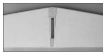
**O** 5. Carefully cut the covering from the bottom of the stab inside the marks you made on the bottom of the stab. Use the same technique for cutting the covering as you used for the wing.
