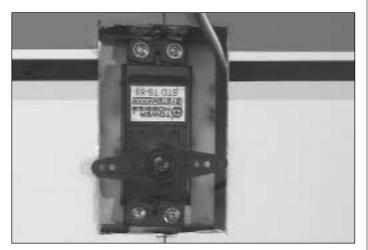
**O** 1. Install your servo into the servo compartment following the instructions included with your particular brand of servo. Install the servo arm in the orientation shown. Drill 1/16" [1.6mm] pilot holes for the servo screws. Remove the servo. Then, install and remove a servo screw into each of the holes. Put a couple of drops of thin CA into each of the holes and
