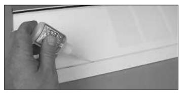
$\bigcirc$   $\bigcirc$   $\bigcirc$  6. Apply six drops of thin CA to the top and bottom of each hinge. Do not use CA accelerator. After the CA has fully hardened test the hinges by pulling on the aileron.
