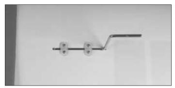
O 3. Locate two nylon landing gear straps and four 2 x 10mm sheet metal screws. Locate the nylon landing gear straps over the landing gear wire. Mark the location for the holes, then drill a 1/16" [1.6mm] hole into the landing gear blocks. Install
