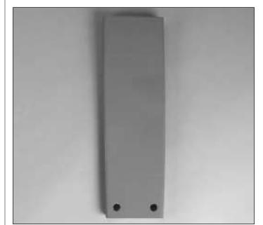
O 12. Locate the **wing belly pan**. Cut the covering away from the holes at the rear of the belly pan.
