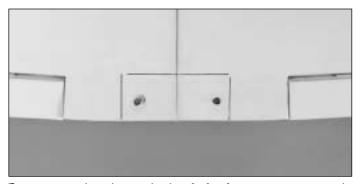
**O** 9. Locate the plywood **wing bolt plate**. Position it on the bottom of the wing over the wing bolt holes. Using a felt tip marker, trace around the wing bolt plate. Using your modeling knife with a sharp blade, cut the covering away, being careful **not to cut** into the surface of the wing skin. Cutting into the wing skin <u>will</u> weaken the structure. The following tip is an alternative method for safely cutting the covering.
