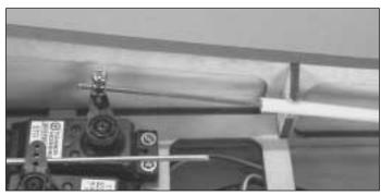
**O** 6. You may find it necessary to shorten the length of the white nylon tube that the throttle pushrod is in. Cut it so that it extends just beyond the former that supports the servo tray. Make a mark on the former at the point where the white nylon tube contacts it. At that point cut a small notch in the former for the tube to rest in. Sand the tube with 220-grit sandpaper where the tube contacts the notch you made in the former. Glue the tube into the notch with 6-minute epoxy.
