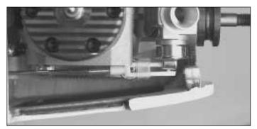
**O** 10. Slide the end of the wire into the tube. Attach the clevis to the throttle arm on the carburetor. Slide the clevis keeper over the clevis.
