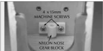
**O** 2. Locate the nylon **nose gear block**. Install it onto the firewall using two  $4 \times 15$ mm machine screws.
