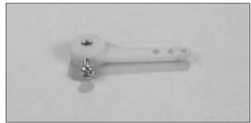
O 6. Install a 4mm wheel collar into the nylon steering arm. Once the wheel collar is in position install a 3 x 10mm machine screw into the arm and wheel collar.
