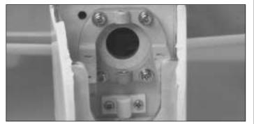
O 3. Install the engine mount to the firewall with four 4 x 15mm machine screws, 4mm lock washers and 4mm flat washers.
