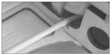
**O** 7. Cut a notch in the former behind the fuel tank for the nose gear steering pushrod tube. Sand the tube with 220-grit sandpaper where the tube rests in the notch you made.
