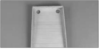
**O** 14. Remove the covering from the edge of the inside of the belly pan. This is most easily done by carefully sanding the edge with a sanding block. Be careful to only sand it as much as needed to remove the covering.
