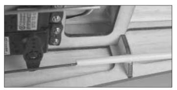
O 8. Cut a notch in the former that supports the servo tray for the nose gear steering pushrod tube.
